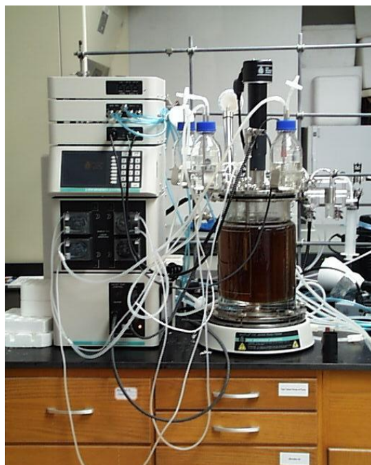
Figure 2.1: Bioreactor used for large scale hemprotein expression. The growth of the transformed E. coli cells to high culture densities was performed using a 5 Liter BioFlo 110 Modular Benchtop Fermentator (New Brunswick, Edison, NJ). A total of 5 L of TB media was supplemented with 30 \mu\text{g}/\text{mL} of chloramphenicol, 70 \mu\text{g}/\text{mL} of kanamycin, and 100 \mu\text{L}/\text{L} of antifoam agent (Sigma, St. Louis, MO). The protein expression was induced by adding 1 mM of IPTG in the mid-log phase ( \text{OD}_{600} , of 1.5–2.0) along with 1 %w/v glucose and 30 \mu\text{g}/\text{mL} hemin chloride. The temperature was maintained at 37 °C before induction and at 30 °C after the addition of IPTG. The culture pH was controlled at 7.0 throughout the process using 1.5 M \text{KH}_2\text{PO}_4 and 30% \text{NH}_4\text{OH} (Sigma, St. Louis, MO). Oxygen supply was maintained a concentration of \text{dO}_2 at 35 % with an agitation cascade of 300-700 rpm. [León et al., 2004; Ramos et al., 2010].
