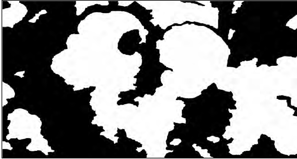
Figure 4.12 Classification of the corals using the supervised merging algorithm on the region growing result of Hurst coefficient/Hough transform
