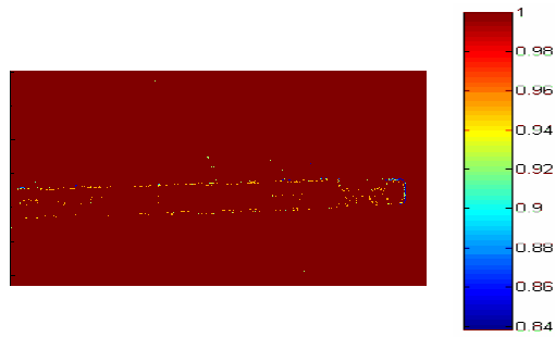
Figure 3.11 Weighted image of Hurst coefficient using the Hough transform of a pencil using a 7x7 circular window.
