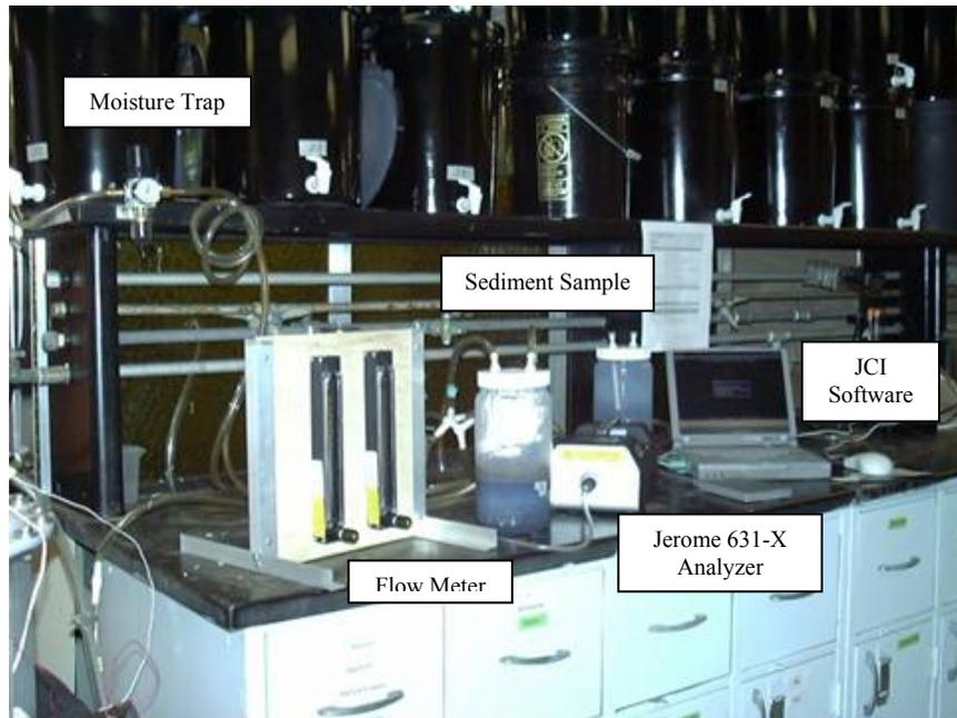
**Figure 8: Set up of the Olfactometry System**
