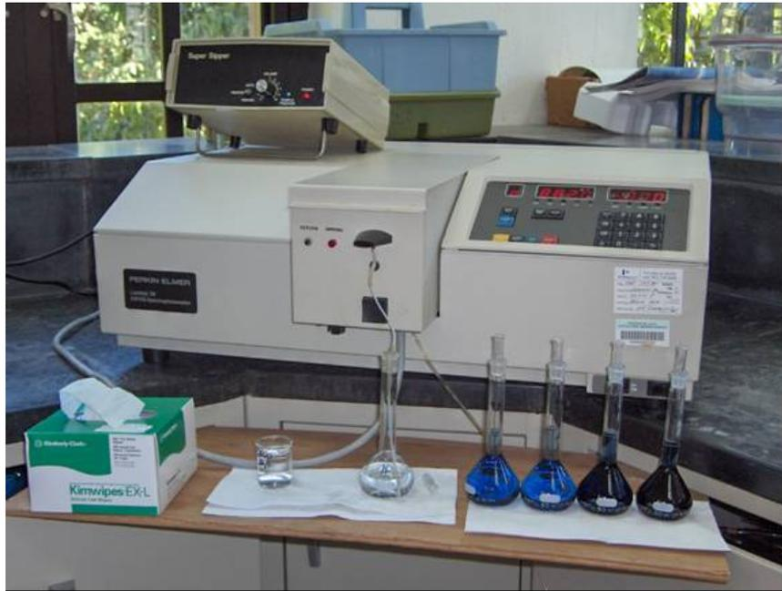
**Figure 7: Perkin Elmer Lambda 3B-UV/VIS Spectrophotometer with a Supper Sipper**
