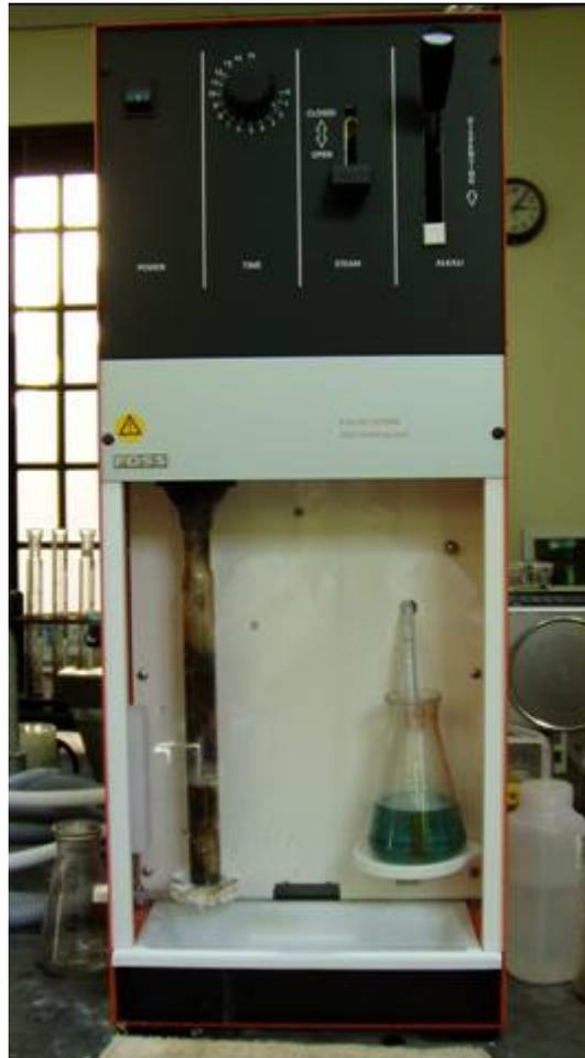
**Figure 6: Kjeltec System-1002 Distilling System with Sediment Sample**
