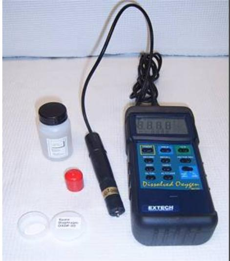
A photograph of an Extech Dissolved Oxygen Meter, Model 407510. The device is a handheld digital meter with a blue display showing '88.88'. It has a black probe connected to the top. Next to the meter are a white plastic bottle with a black cap, a red cap, and a small white container with a label that reads 'Heavy Duty Dissolved Oxygen Meter Model 407510'.                      | D             |
