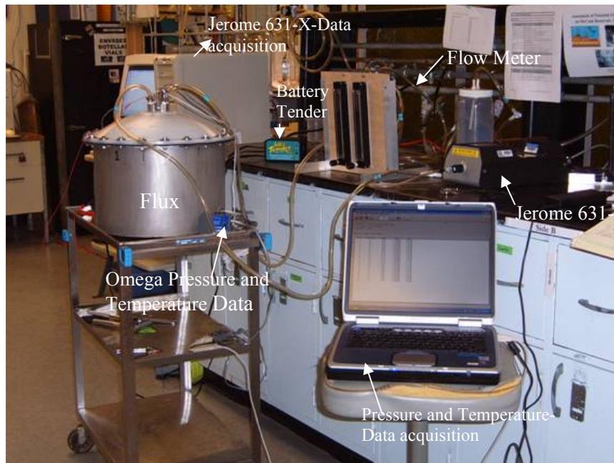
**Figure 15: Flux Chamber Test**
