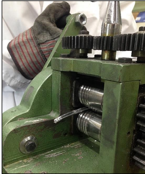
Figure 3.6 Cold rolling process of the cylindrical ingots.
