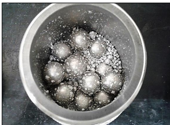
Figure 3.4 Nanocomposite pellets inside the jars after cold welding.
