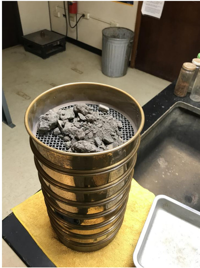
Figure 5.3. Soil sample MC2 placed on the stack of sieve prior to shacking of the sample.
