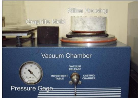
Figure 15 Front view of the adapted vacuum equipment.
