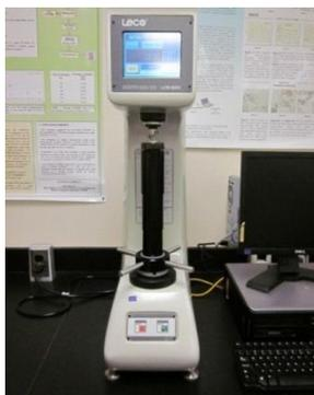
Figure 18 LECO Rockwell LR-50 hardness tester.
