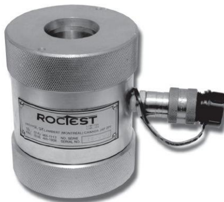
Figure 3-9: Hoek triaxial cell (left); rubber membrane with U-shaped end seals (right)
