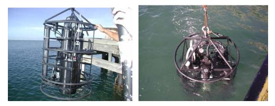
Figure 3. CTD/rosette instrument to measure temperature, conductivity, fluorescence, transmissivity, and water samples for pH, salinity, and dissolved oxygen.
