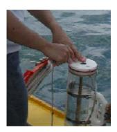
Figure 4. Bailer sampler used for water collection at 10 ft.
