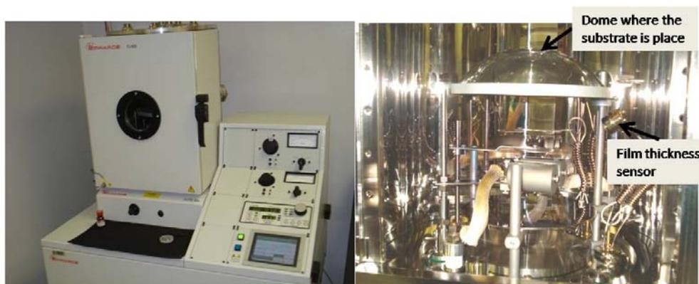
**Figure 4-3:** Picture of the EDWARDS FL 400/AUTO 306 Physical Vapor Deposition (PVD) system used to evaporate silver over the nanostructured polymer.
