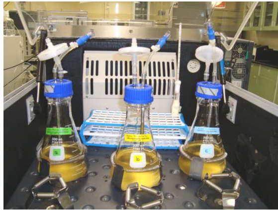
Figure 3.3 - Batch fermentation in an Innova 4000 incubator shaker.
