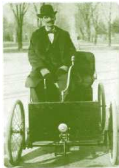
Figure 2.1 – Ford Model Car (1896), which used pure ethanol [5].
