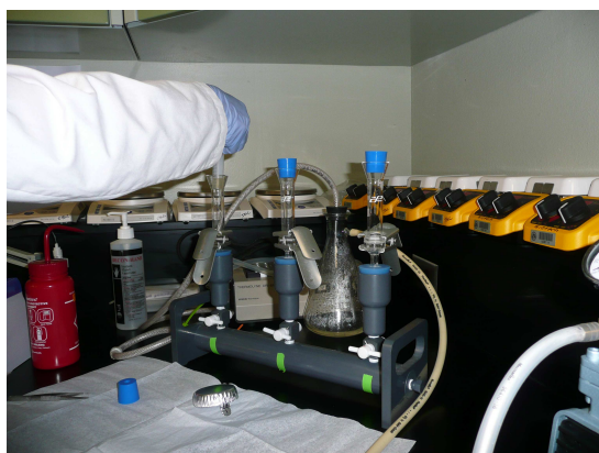
Figure 3.5 - Manifold filtration unit used for cell filtration.
