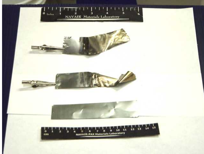
Figure 4.35 Macroscopic deformation during hydrogen charging on the AISI-321SS steel [56]
