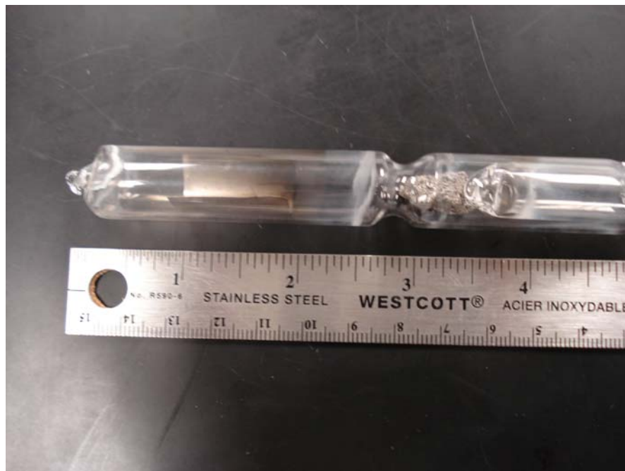
Figure 3.2 Quartz vacuum ampoule employed for AISI321 samples heat treatment
