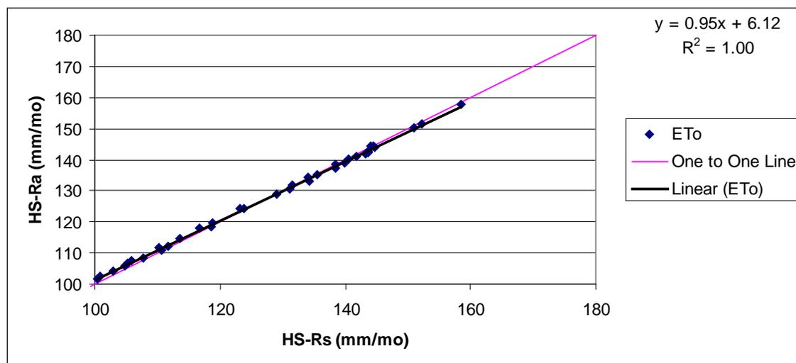
Figure A.1. Hargreaves Samani from measured solar radiation ( $R_s$ ) vs Hargreaves Samani from average extraterrestrial radiation ( $R_a$ ).
