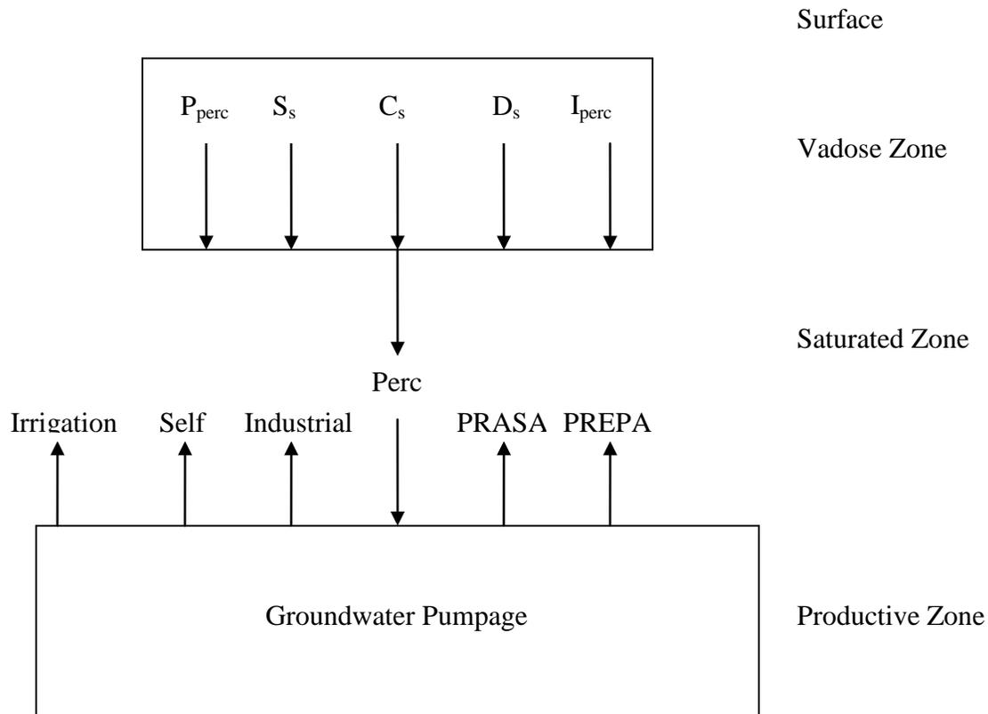
Figure 23. Conceptual model of the monthly groundwater balance for each water-budget area in the Salinas to Patillas region.
