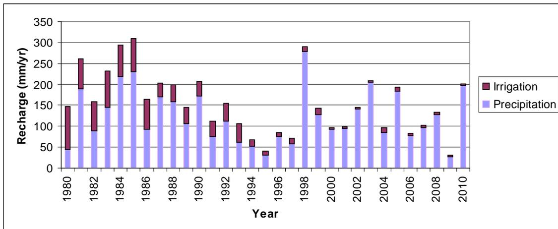
Figure 62. Estimated annual percolation that serve as recharge from precipitation and irrigation for Salinas modeling area.
