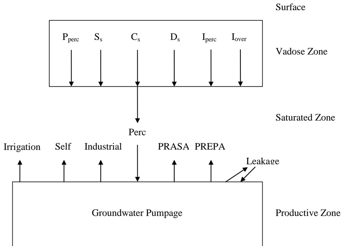
Figure 24. Conceptual model of the annual groundwater balance for each water-budget area in the Salinas to Patillas region.
