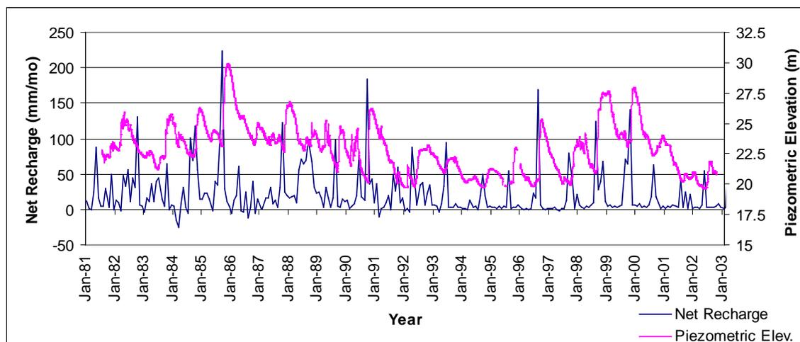
Figure 83. Estimated changes in storage represented by net recharge estimates compared to piezometric elevations for the Juana well as measured daily in Guayama, 39 m surface elevation.
