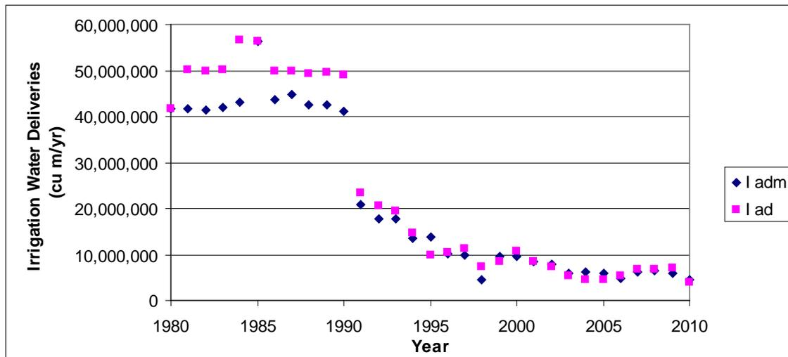
Figure A.6. Annual irrigation surface water deliveries (I ad) as compared to the sum of estimated annual surface water deliveries by sub-modeling area.
