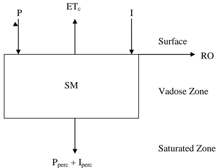
Figure 21. Conceptual model of the daily soil moisture balance for each water-budget area in the Salinas to Patillas region.
