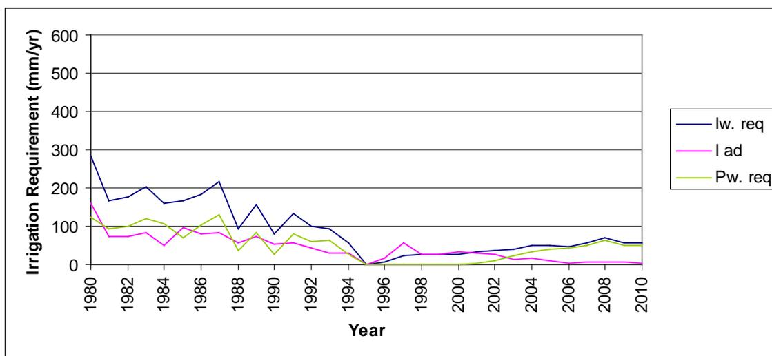
Figure A.8. Irrigation water requirement (Iw. req), imports (I ad) and extractions (Pw. req) for Arroyo modeling area
