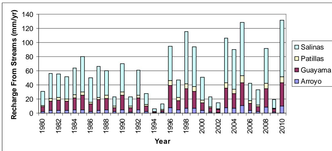
Figure 89. Estimated recharge from stream base flow percolation for the Irrigated Watersheds modeling area.
