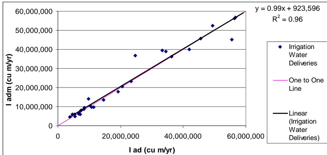
Figure 33. Yearly product from estimated monthly irrigation water deliveries ( $I_{adm}$ ) from 1981 through 1989 compared to those published by Quiñones-Aponte et al., (1997) referred as  $I_{ad}$ .
