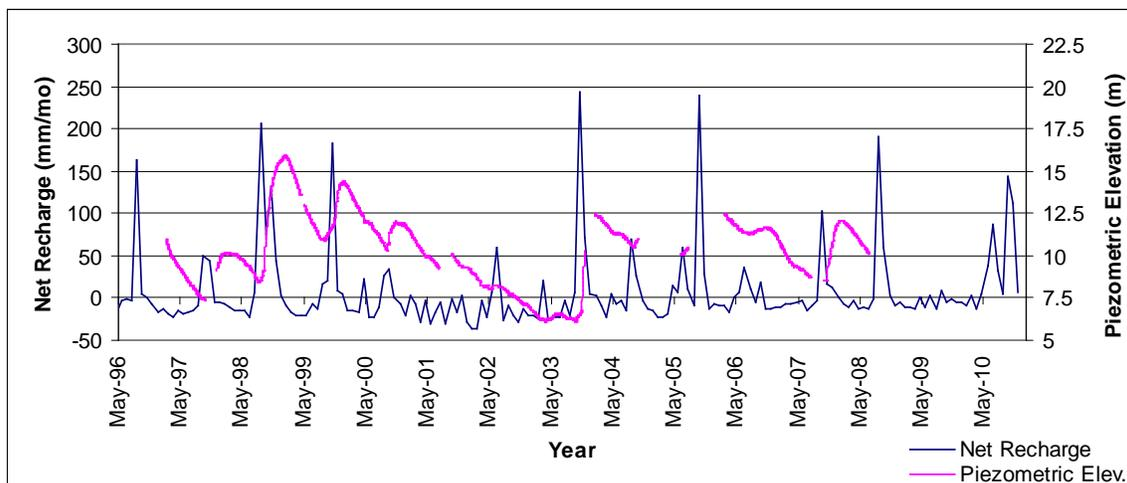
Figure 81. Estimated changes in storage represented by net recharge estimates compared to piezometric elevations for the Rasa D well in Salinas as measured daily, 27.4 m surface elevation.
