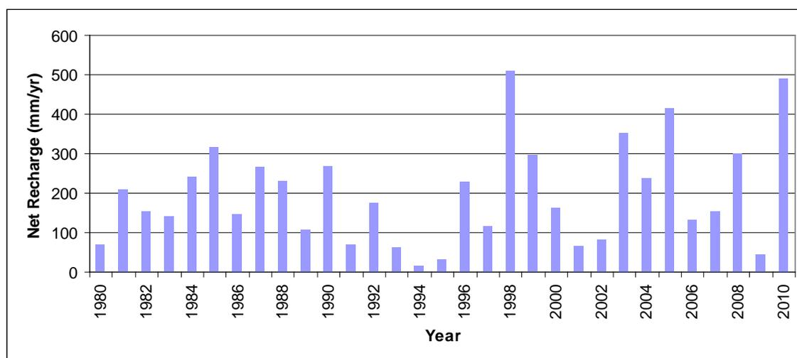
Figure 101. Case scenario where no groundwater pumpage for irrigation purposes take place and all irrigation water is retrieved from canals, based on an extrapolation of today's irrigation conditions to historical data.
