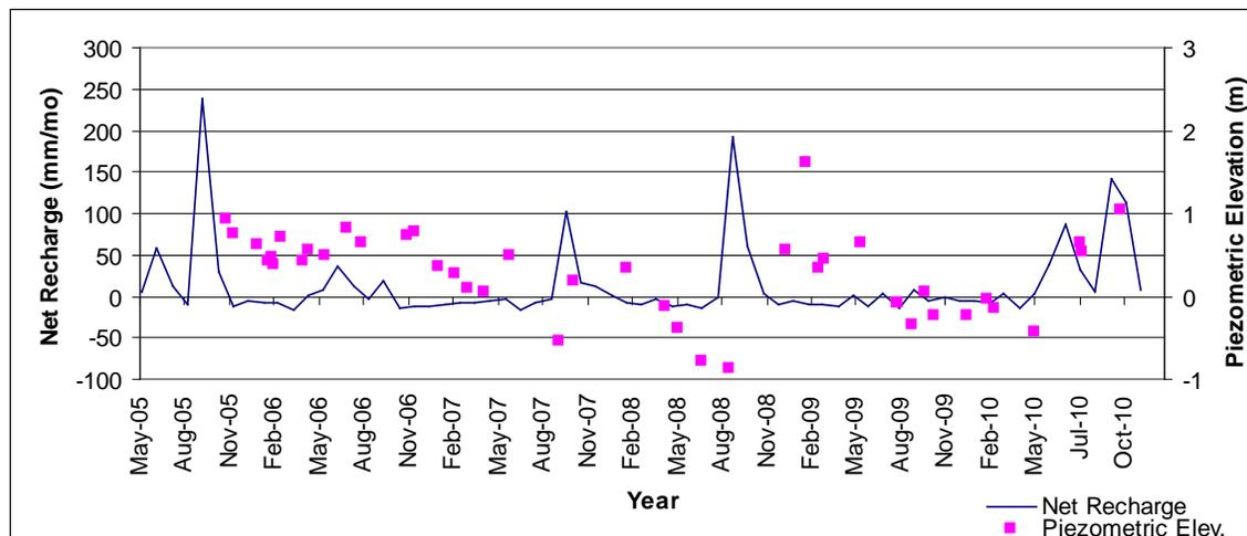
Figure 79. Estimated changes in storage represented by net recharge estimates compared to piezometric elevations for the JBNERR east 2 well in Salinas as measured periodically, 1.5 m surface elevation.
