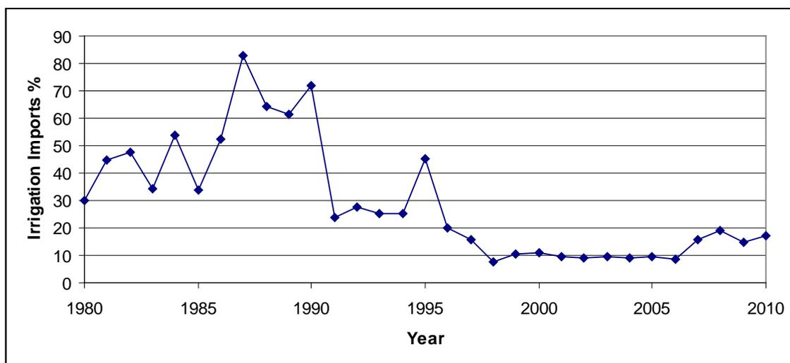
Figure 100. Changes in irrigation water imports to farms for irrigation by PREPA as a fraction of irrigation water requirement for Salinas modeling area.
