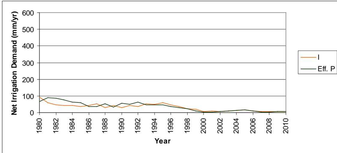
Figure A.11. Net irrigation water demand (I) and effective precipitation (Eff. P) for Patillas modeling area
