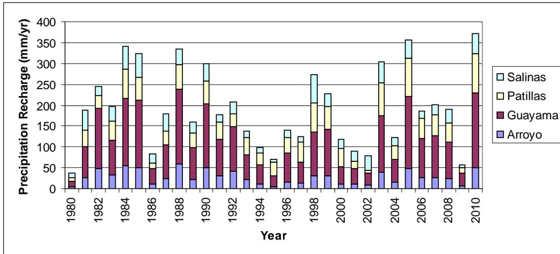
Figure 88. Estimated recharge from precipitation percolation for the Irrigated Watersheds modeling area.
