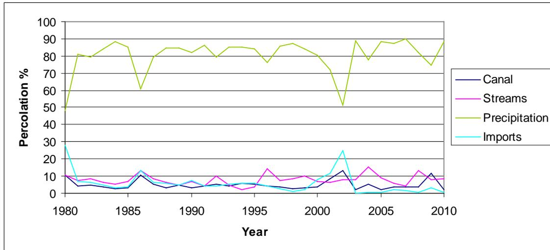
Figure 98. Relative importance of each percolation factor to aquifer recharge for the Patillas modeling area in an annual basis.
