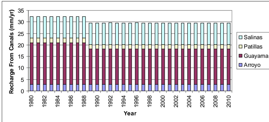
Figure 90. Estimated recharge from irrigation canals percolation for the Irrigated Watersheds modeling area.
