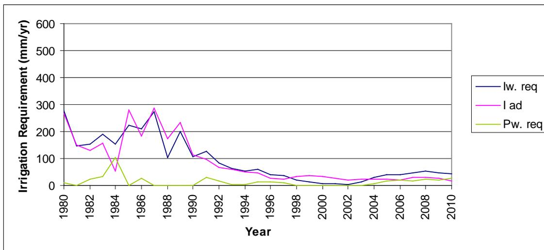
Figure A.10. Irrigation water requirement (Iw. req), imports (I ad) and extractions (Pw. req) for Guayama modeling area
