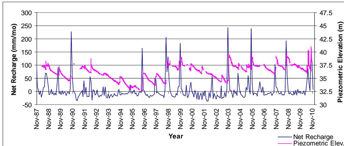
Figure 82. Estimated changes in storage represented by net recharge estimates compared to piezometric elevations for the Aguirre well in Salinas as measured daily, 41.2 m surface elevation.
