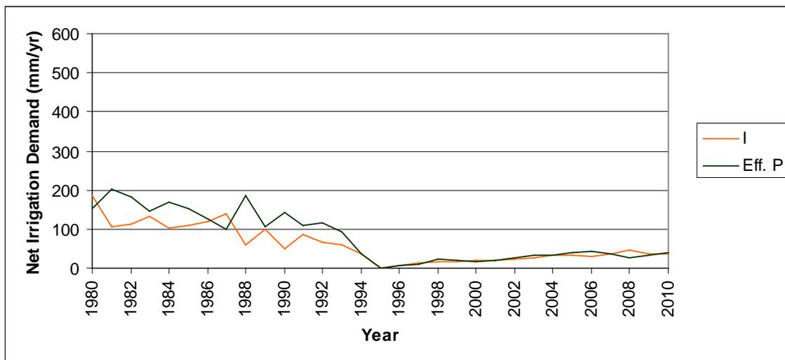
Figure A.7. Net irrigation water demand (I) and effective precipitation (Eff. P) for Arroyo modeling area
