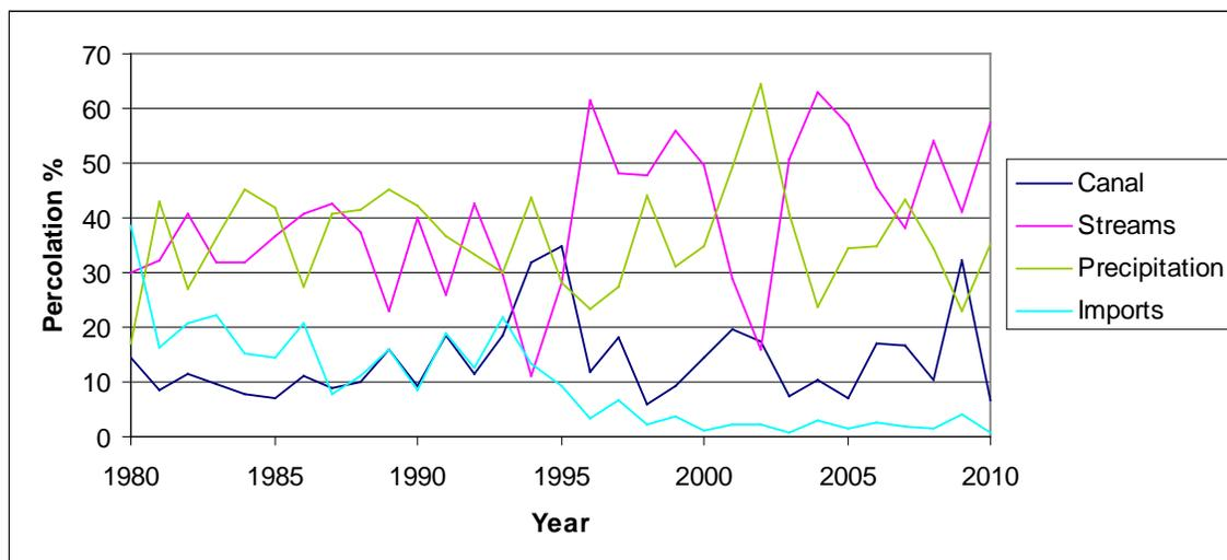
Figure 99. Relative importance of each percolation factor to aquifer recharge for the Salinas modeling area in an annual basis.
