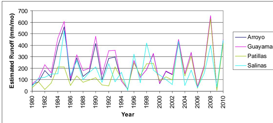
Figure 58. Estimated annual runoff based on the SCS CN method per modeling area.
