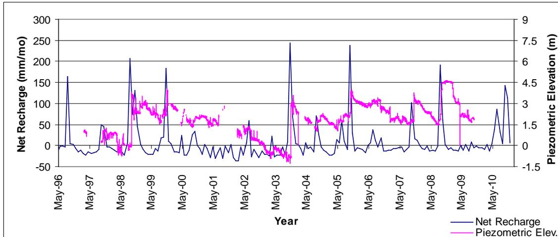
Figure 80. Estimated changes in storage represented by net recharge estimates compared to piezometric elevations for the Coquí well in Salinas as measured daily, 4.9 m surface elevation.
