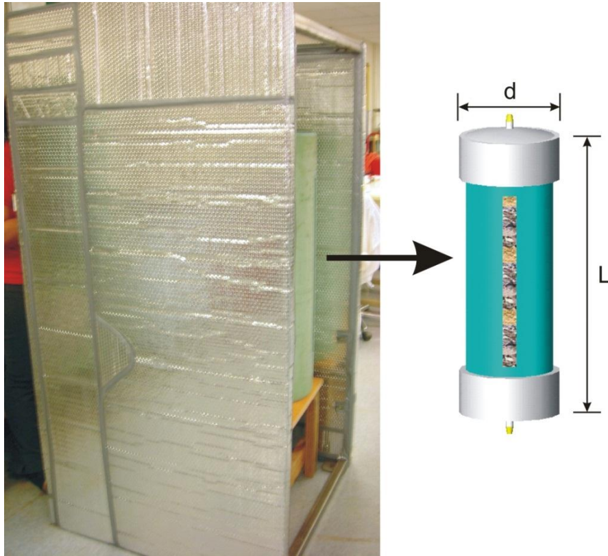
Figure 10 Environmental Chamber and Physical Landfill Model.
