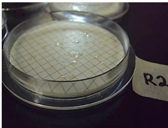
Figure 78 Heterotrophic Plate Count with a Membrane Filtration for the Reactor 2 (5.0 g CCAs/L) ( 10^{10} Dilution).
