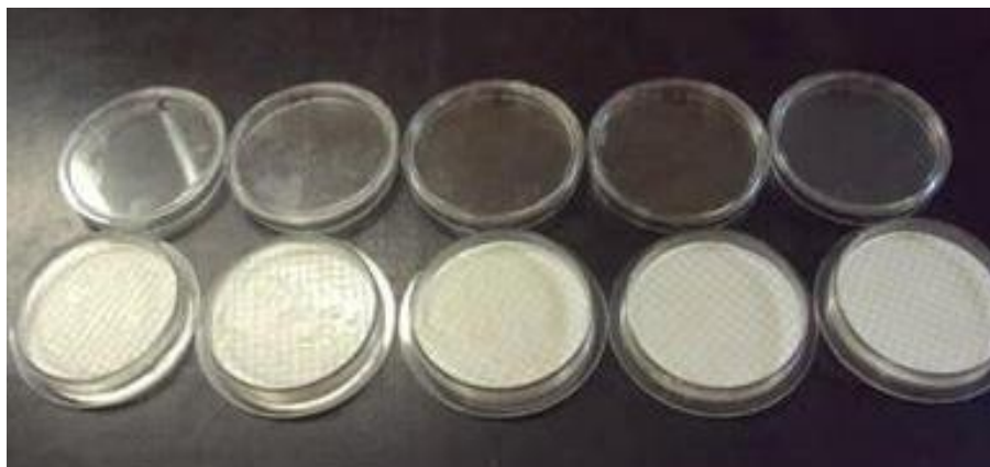
Figure 75 Heterotrophic Plate Count with a Membrane Filtration (Dilution was 10^4 for Control and 10^6 for others).
