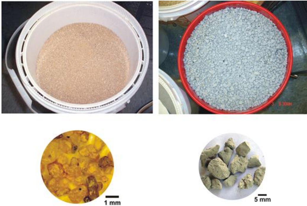
Figure 4 Sand and CCAs Used for Daily Covers in this Study.
