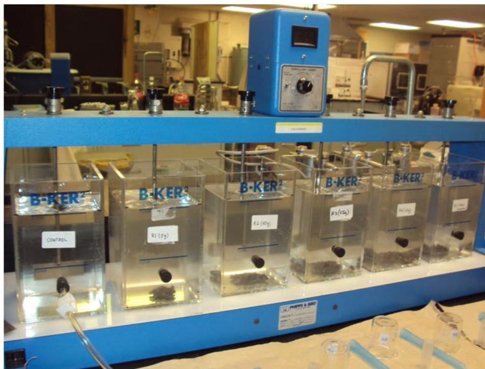
Figure 14 Jar Test Used in the Experiment.
