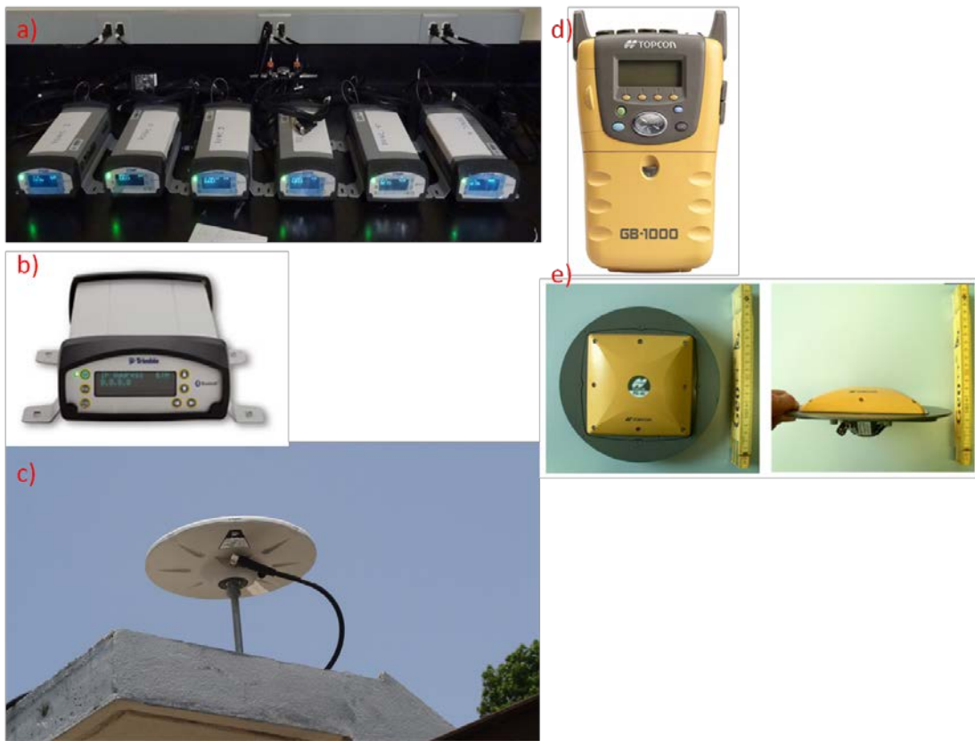
Figure 3-2: Equipment used to monitor the Cerca del Cielo community. The left column shows Trimble's NetR9 receivers (a), Trimble's NetR8 ( www.trimble.com ) receivers (b) and Trimble Zephyr-Geodetic Model 2 antennae (c). The right column shows the Topcon's GB-1000 ( www.topconpositioning.com ) receiver (c) and Topcon's PG-A1 ( www.unavco.org ) antennae (d).
