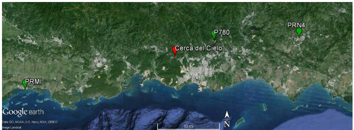
Figure 3-6: NGS CORS GPS stations (green markers) from the CORS used as reference to monitor the Cerca del Cielo community (red marker) (Google Earth©).
