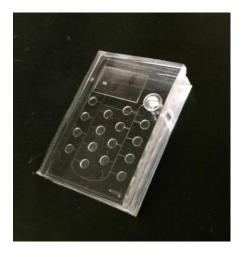
Figure 4: Quick Chip design cast in PDMS
