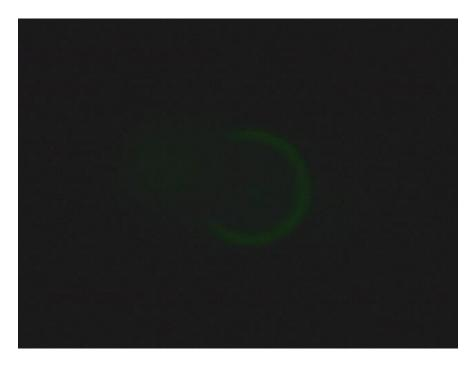
*Figure 8: 500 nM 6-fam sample on acrylic slide.* Two fluorescent signatures are present from a single droplet of sample. The dimmer one on the right was the sample as excited from the bottom. The second signal was the reflection on the excitation filter.
