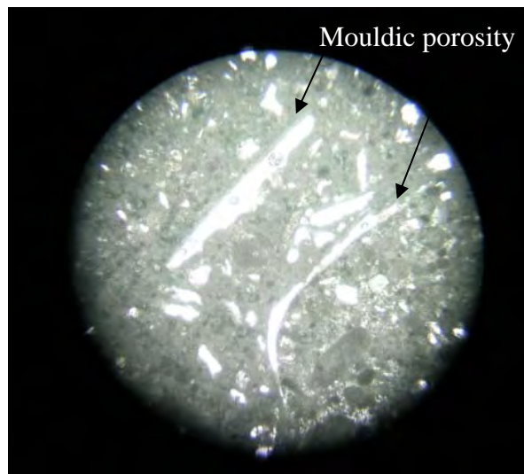
Figure 4.5: Picture of thin section from NC-10 7.9 m showing mouldic porosity.
