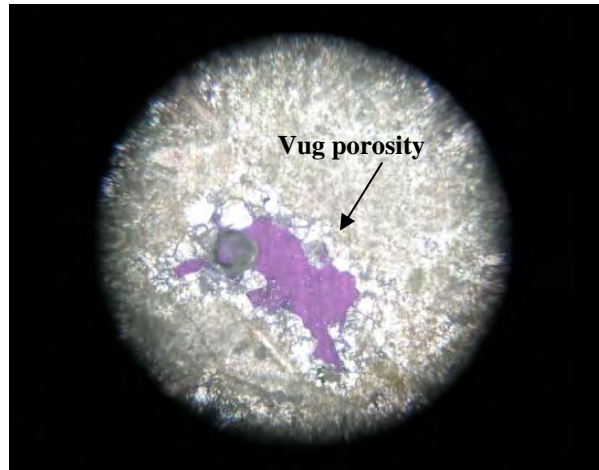
Figure 4.2: Picture of thin section from NC-4 32.3 m showing vug porosity.
