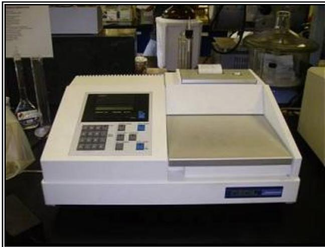
**Figure 3-4: Picture of the Cecil® 3000 Series Scanning Spectrophotometer**
