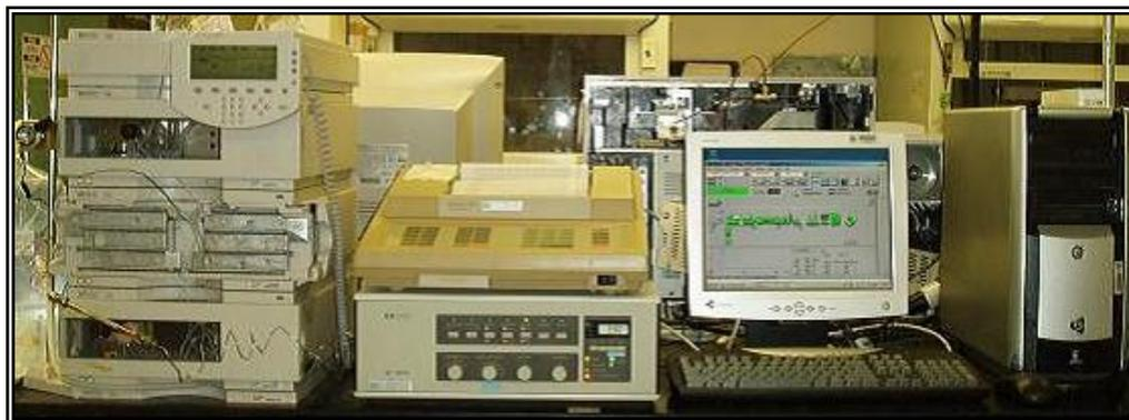
**Figure 3-3: Picture of the Hewlett Packard Series 1100 High Performance Liquid Chromatograph**
