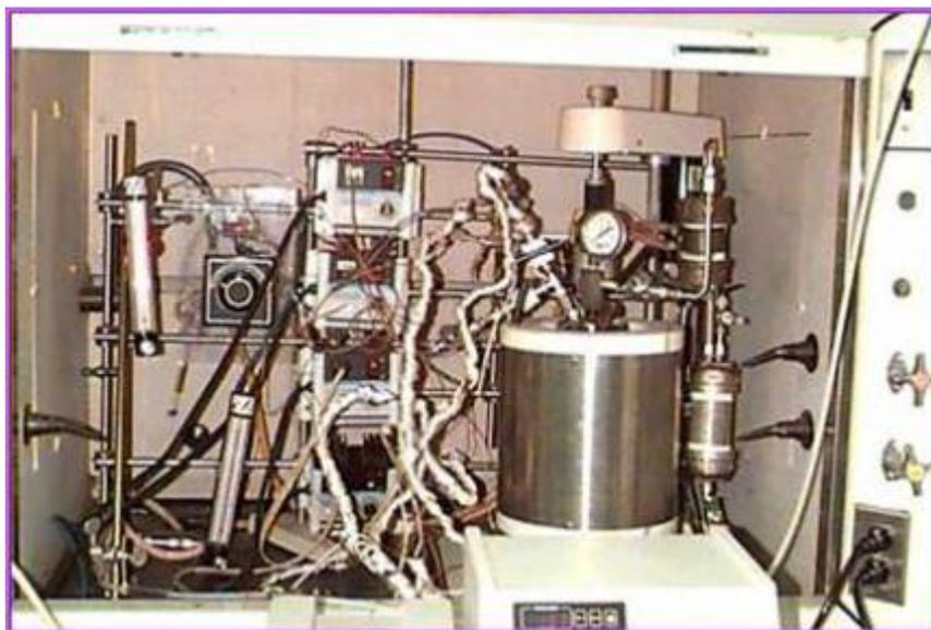
Figure 3.2. The Bench Stirred Tank Reactor (BSTR) system.
