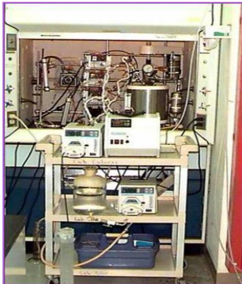
Figure 3.5. The BSTR system including the peristaltic pumps and the temperature controller.
