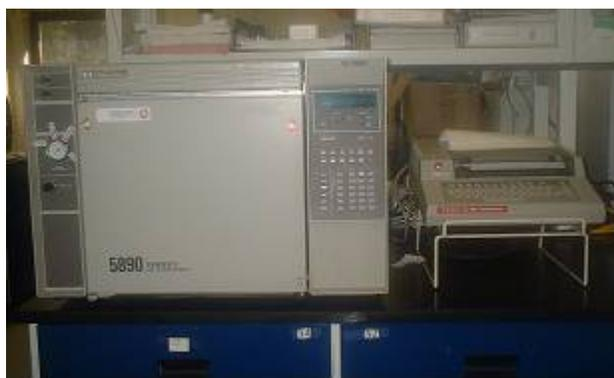
Figure 3.6. Gas Chromatograph-TCD with the Integrator
