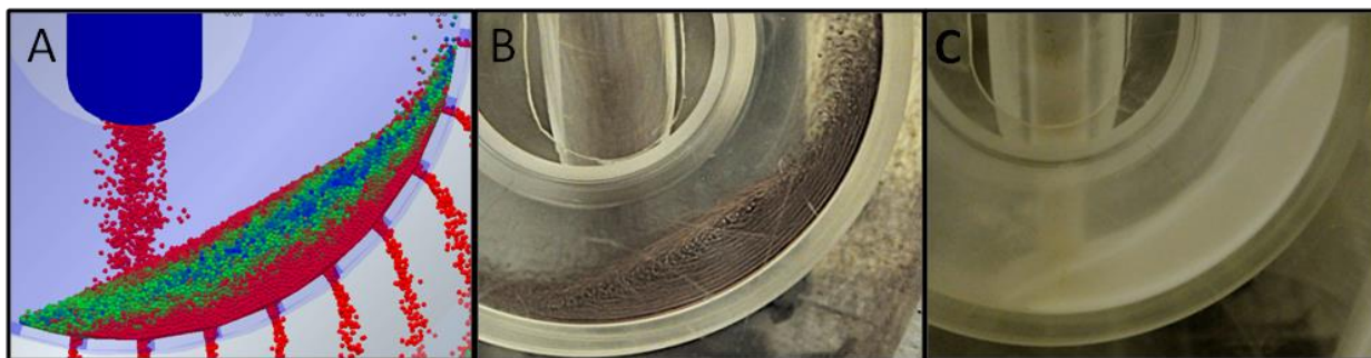
Figure 4.6. Simulation and validation using lactose and glass beads at 70 RPM.
