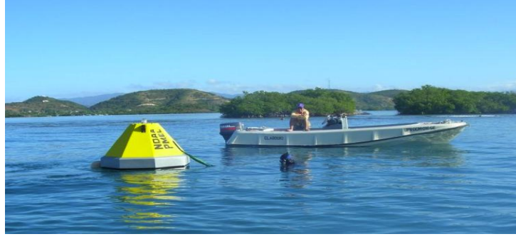
Figure 2: The MapCO 2 buoy deployed at Enrique mid shelf reef provides measurements of atmosphere and seawater CO 2 mole fraction, seawater temperature and salinity at 3-hour intervals (photo by Gledhill, D.).
