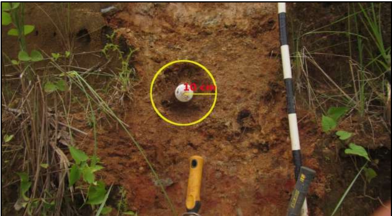
Figure 14: Sampling tube in site RC-7. Circle shows area where dose rate and water content samples were taken.
