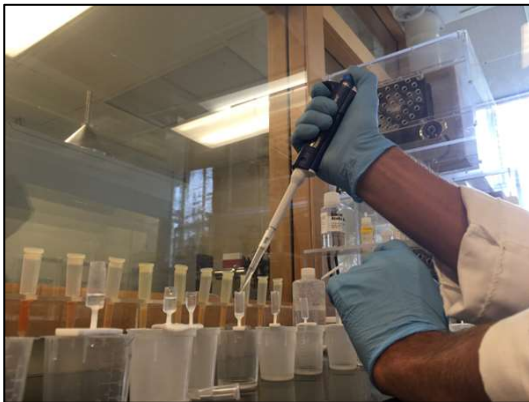
Figure 27: Strontium separation via column chemistry at the Geochronology Isotope Geochemistry Lab, UNC Chapel Hill. Sr was separated using Sr specific rosin. The rosin works by preferentially bonding with Sr ions under certain condition and will release the bound ions once rinsed with H_2O
