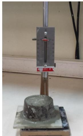
**Figure 5. Vicat needle used to measure setting time**
