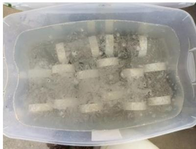
**Figure 9. PCPC specimens (C-2 design) in reservoir with 0.1% H<sub>2</sub>O<sub>2</sub> solution**
