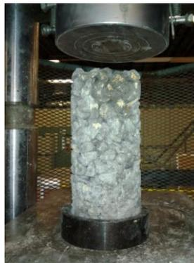
**Figure 6. PCPC being tested for compressive strength**
