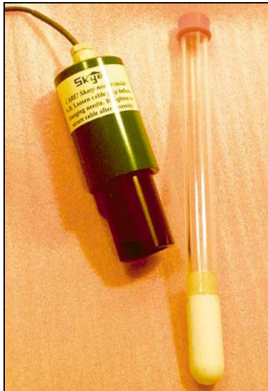
Figure 5.2 Septum tensiometer with needle sensor.
