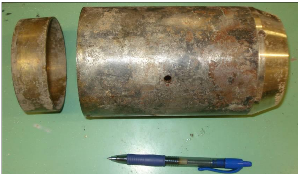
Figure 5.13 Sampler with cylinder used to collect samples for Tempe Pressure Cell.
