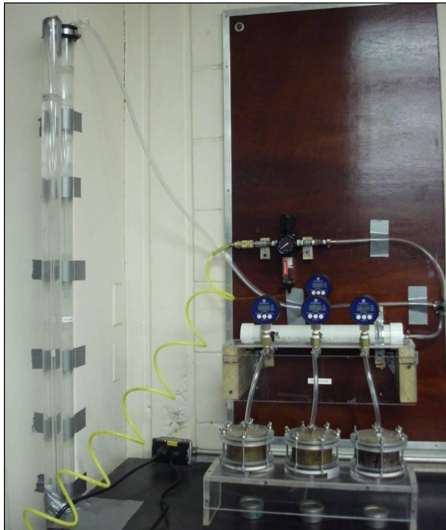
Figure 5.12 Test set-up for soil-water characteristic curve determination.
