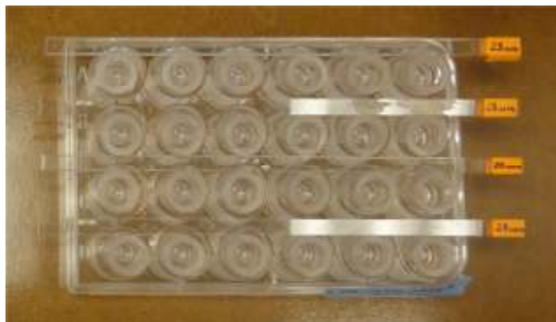
Figure A-1. 2: Migration plate used for LMIA. The plate consists of a 24 well tissue culture plate with 4 migration racks, each of these composed of 6 circular plexiglass tubes with a 28 \mu\text{m} mesh glued to the bottom.
