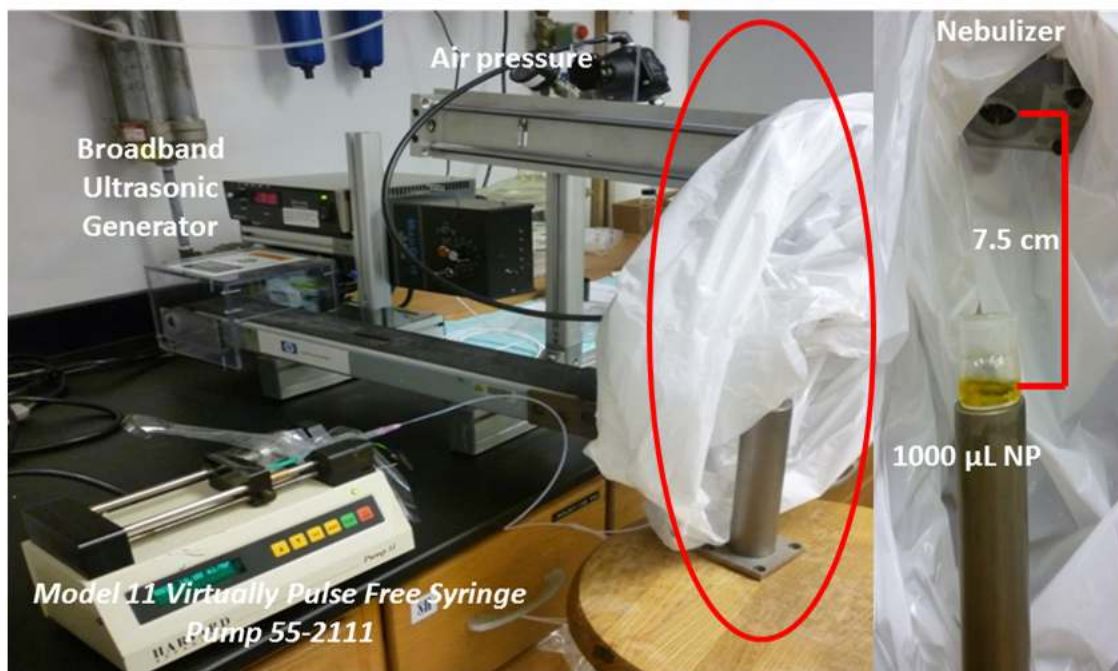
Figure 45. Experimental setup used to aerosolize the bacterial sample to the nanoparticles for SERS experiments. The parameters used were 50 mL/h, 1.5 atm at 0.10 of broadband speed.
