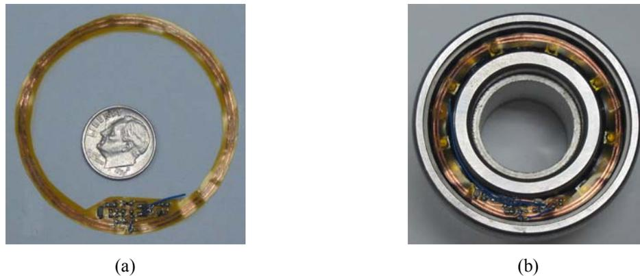
Figure 1. Remotely powered wireless temperature sensor (a) Printed circuit implemented (b) bearing instrumented with the sensor
