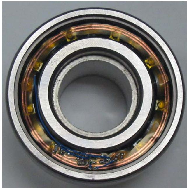
Figure 41. RF-powered wireless temperature sensor based on LC Colpitts oscillator installed on a ball bearing built over a polyimide film
