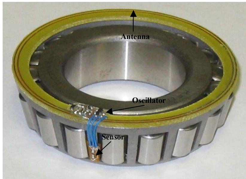
Figure 40. Latest version of the RF-powered wireless temperature sensor based on LC Colpitts oscillator installed on a tapered roller bearing
