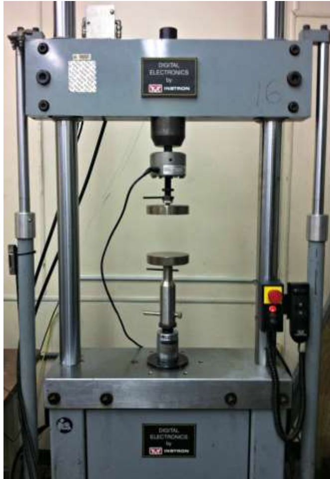
Figure 44: MTS compression test machine.
