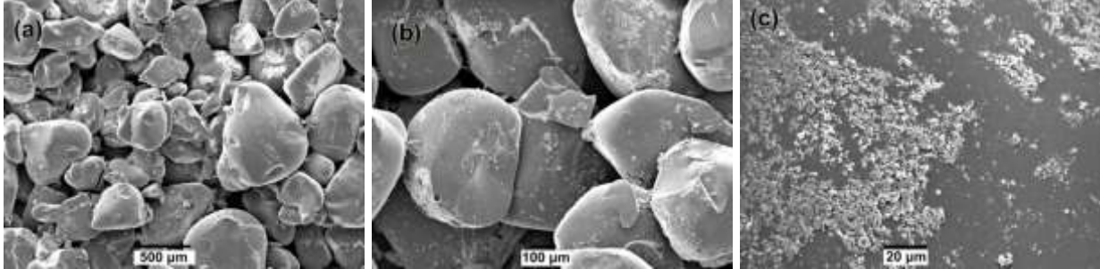
Figure 22: SEM images of MG30 recycled glass beads mixed with 1% TiO 2 sintered at 800°C for 20 minutes, (a) 500 μm, (b) 100 μm, (c) 20 μm.
