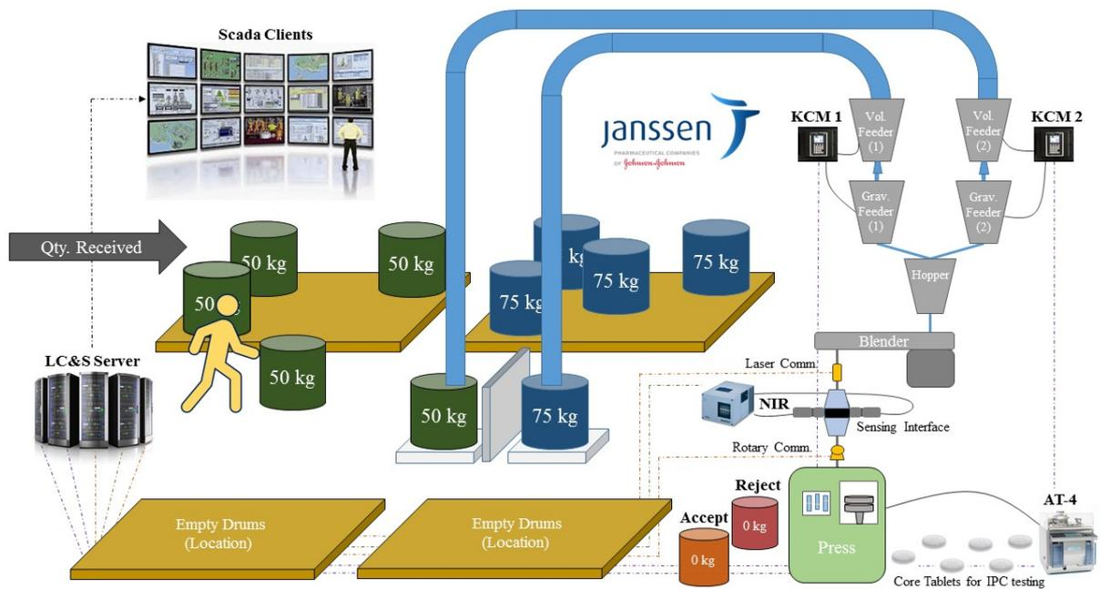
**Figure 5.3:** Schematic Representation of the CM line
