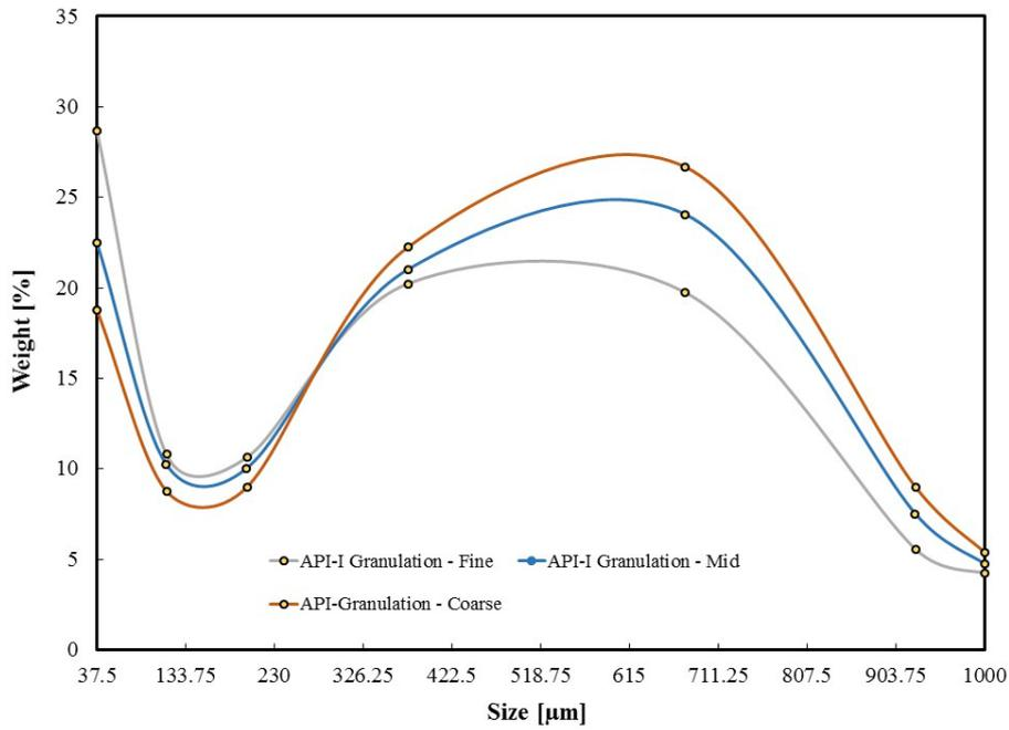
**Figure 3.1:** API-I Granulation PSD from Niro FBG/D unit operation
