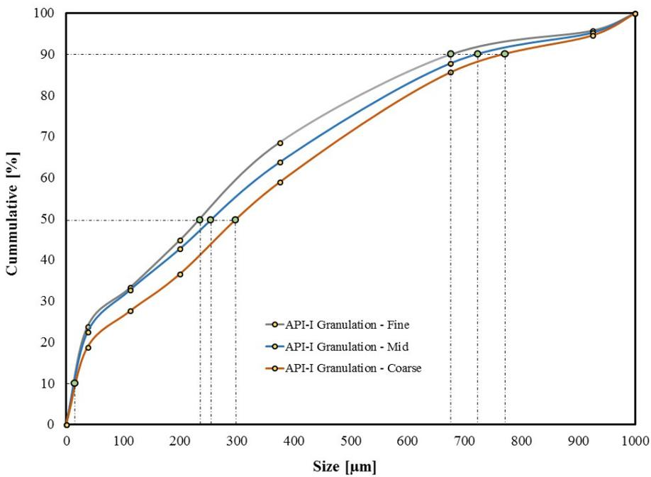
**Figure 3.2:** API-I Granulation Cumulative from Niro FBG/D unit operation
