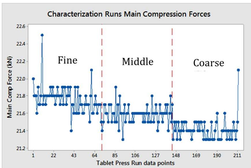
**Figure 4.12:** Main Compression (factor) Force from the Korsch Tablet Press
