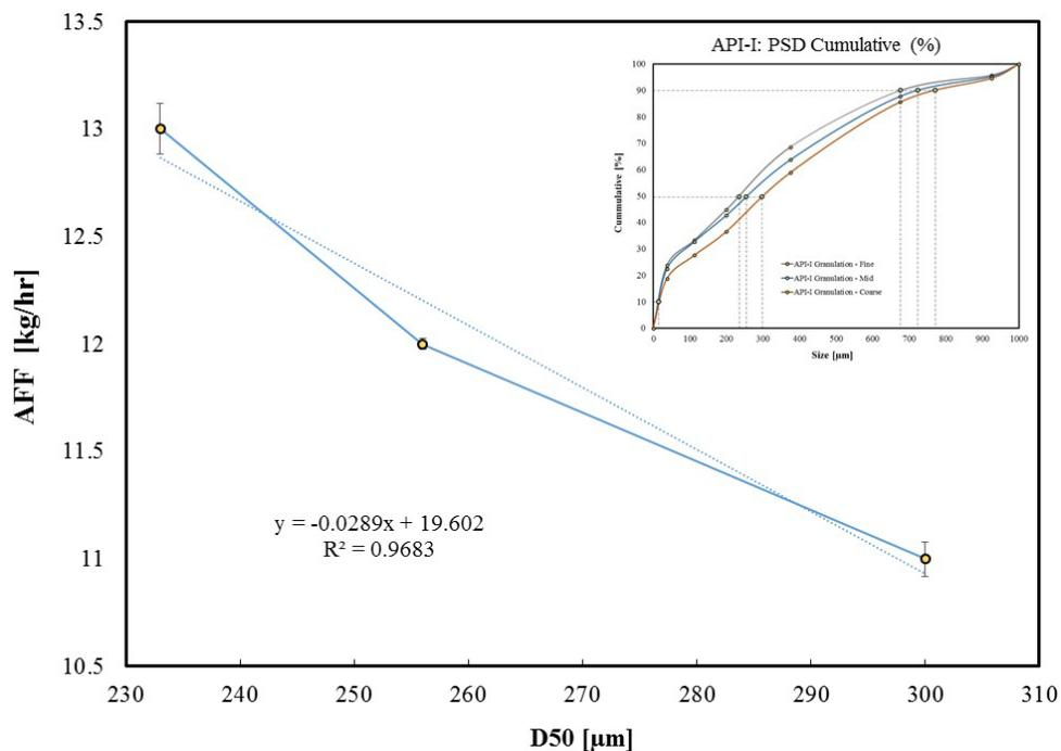
**Figure 4.7:** Linear Regression - Average Feed Factor vs API granulation PSD
