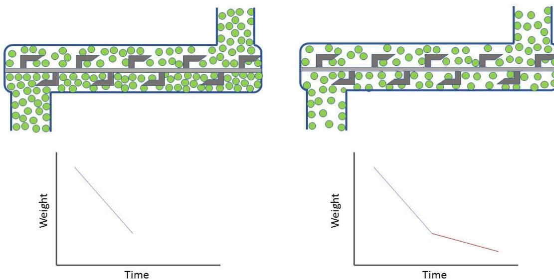
**Figure 2.2:** Screw Fill vs Weight Loss rate correlation
