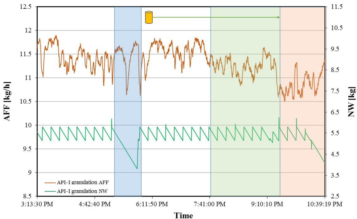
**Figure 4.13:** Control Experiment Trend Base on API-I Granulation Feeder Netweight [kg] and Average Feed Factor [kg/h] for the 50/1000 mg FDC
