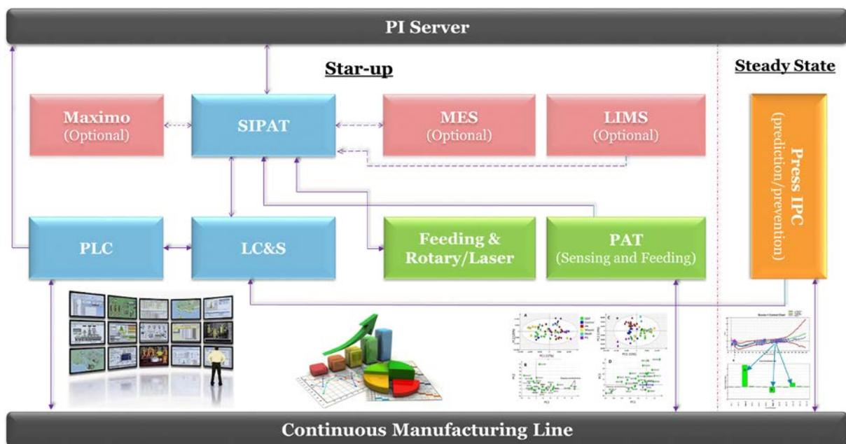
**Figure 5.2:** Schematic Representation to Connect Historian and Data Bases Software for Robust Data Analysis Through the Search of CM Line Elements and Material Properties Interaction
