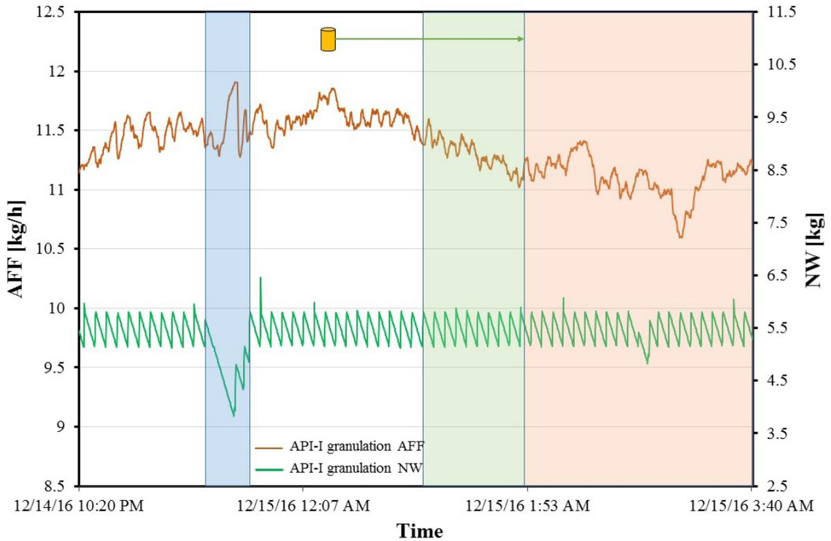
**Figure 4.14:** Control Experiment Trend Base on API-I Granulation Feeder Netweight [kg] and Average Feed Factor [kg/h] for the API-I 150/1000 mg FDC
