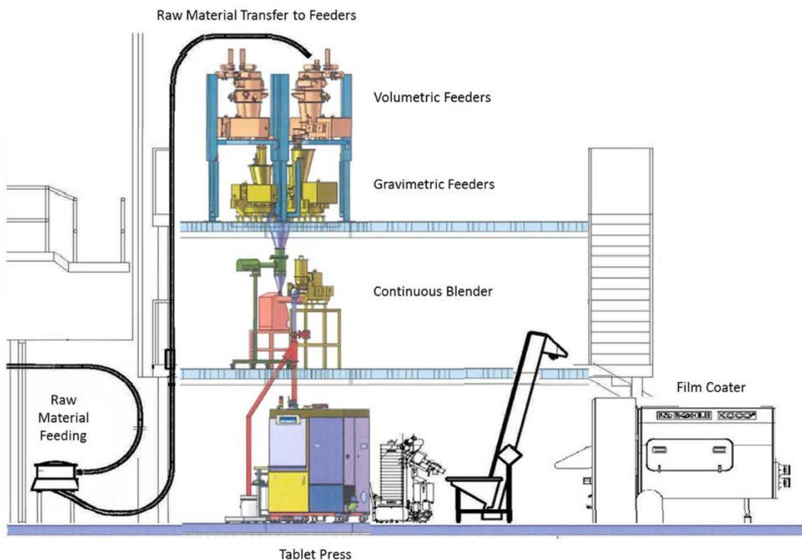
**Figure 3.3:** Schematic representation of the CM line
