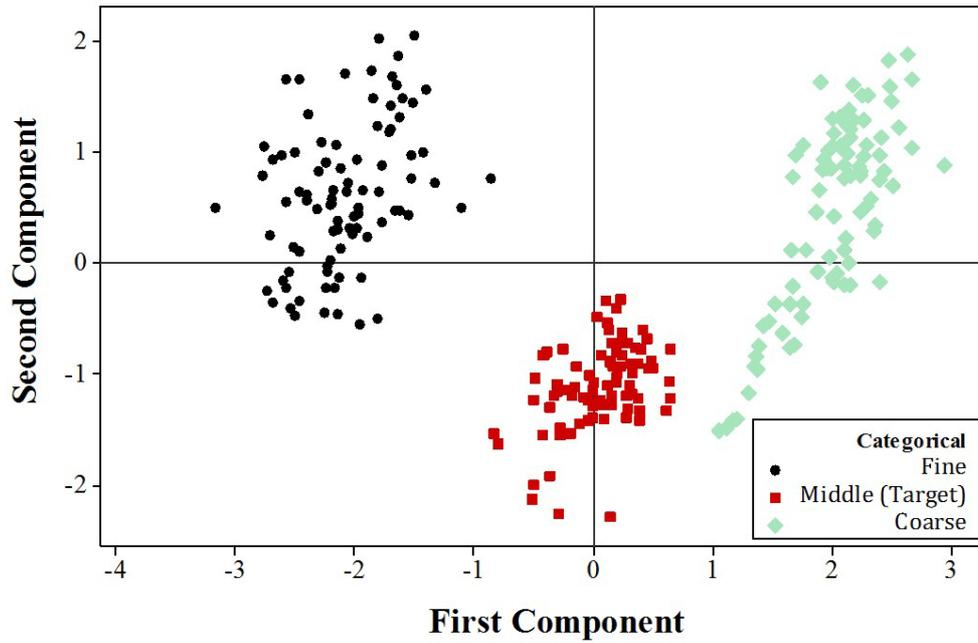
**Figure 4.3:** Score Plot from Drive Command (DC), Motor Speed (MS) and Average Feed Factor (AFF)
