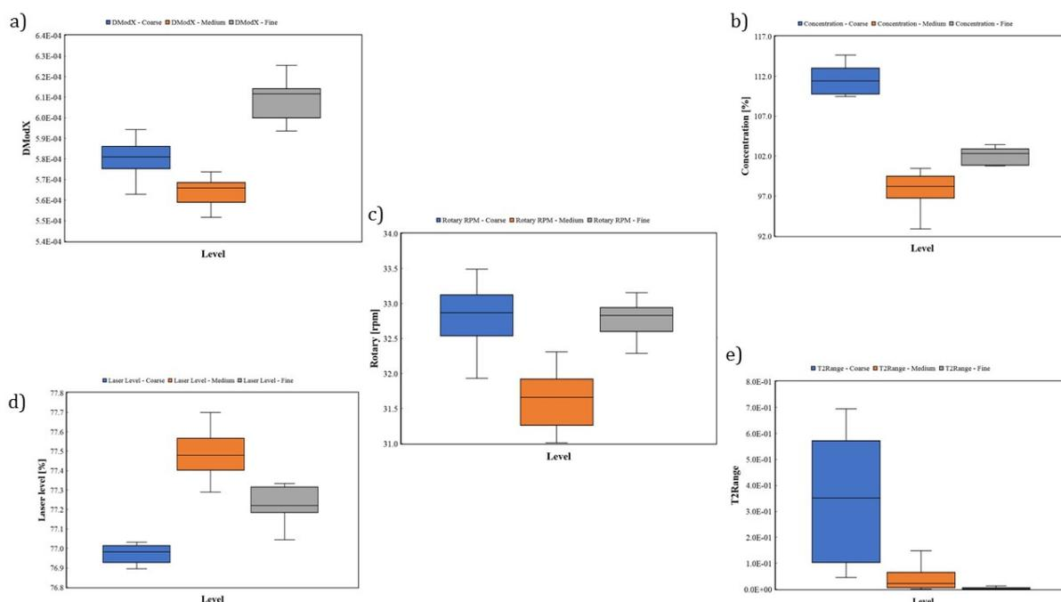
**Figure 4.11:** Box plot of a) DModX b) API-I Concentration c) Rotary RPM d) Laser Level and e) T2Range vs the Three (3) API-I Granulation: Coarse, Medium and Fine
