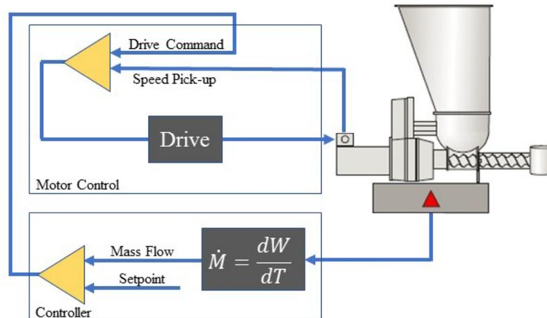
**Figure 2.1:** Schematic representation of feeder control logic for feeding performance.
