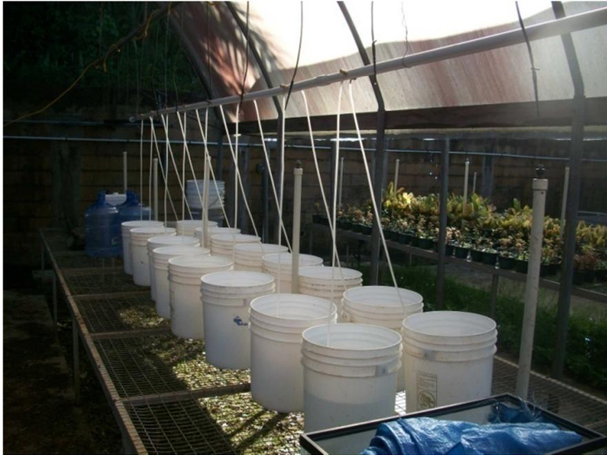
Figure 3.1. The experimental set-up. Each bucket represents a mesocosm. The transparent tubes represent the aeration system. At the top of the picture, the clear covering is visible which allows sunlight to penetrate but not rain.
