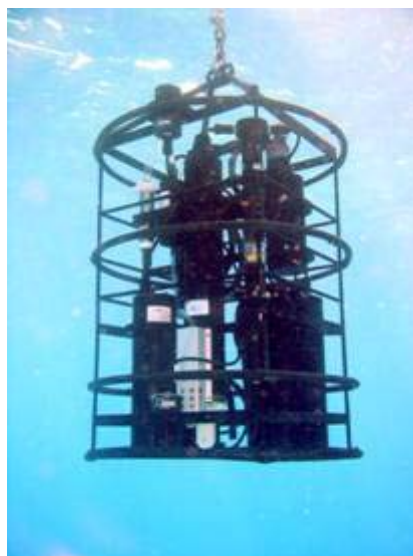
Figure 4c. Bio- Optical package containing CTD, fluorometer, AC-9 and a Hydroscat-6.
