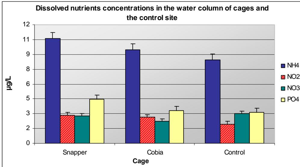
Figure 8. Dissolved nutrients concentrations ( $\mu\text{g/L}$ ) of ammonia-N ( $\text{NH}_4$ ), nitrate-N ( $\text{NH}_3$ ), nitrite-N ( $\text{NH}_2$ ) and phosphate ( $\text{PO}_4$ ) in the water column for each cage and control sites.
