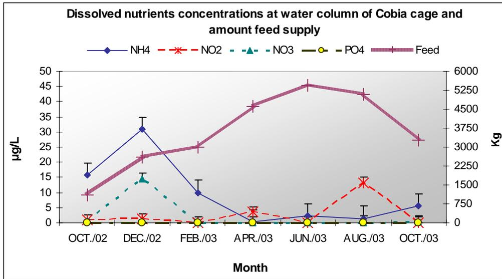
Figure 25. Temporal variation of dissolved nutrient concentrations ( $\mu\text{g/L}$ ) of ammonia-N ( $\text{NH}_4$ ), nitrate-N ( $\text{NH}_3$ ), nitrite-N ( $\text{NH}_2$ ) and phosphate ( $\text{PO}_4$ ) in the water column of the *R. canadum* (cobia) cage compared with feed supply ( $\text{kg/month}$ ).
