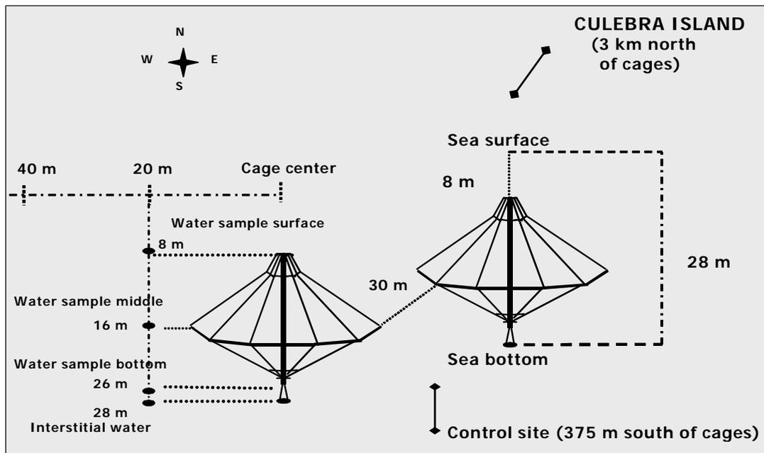
Figure 5. Diagram of the Sea Station™ culture cages and sampling locations in the water column.
