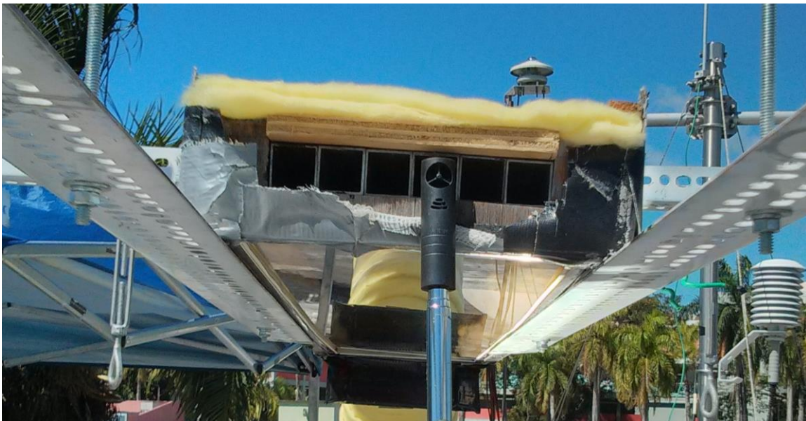
Figure 39: Measuring the inlet of the tubes with an anemometer probe.
