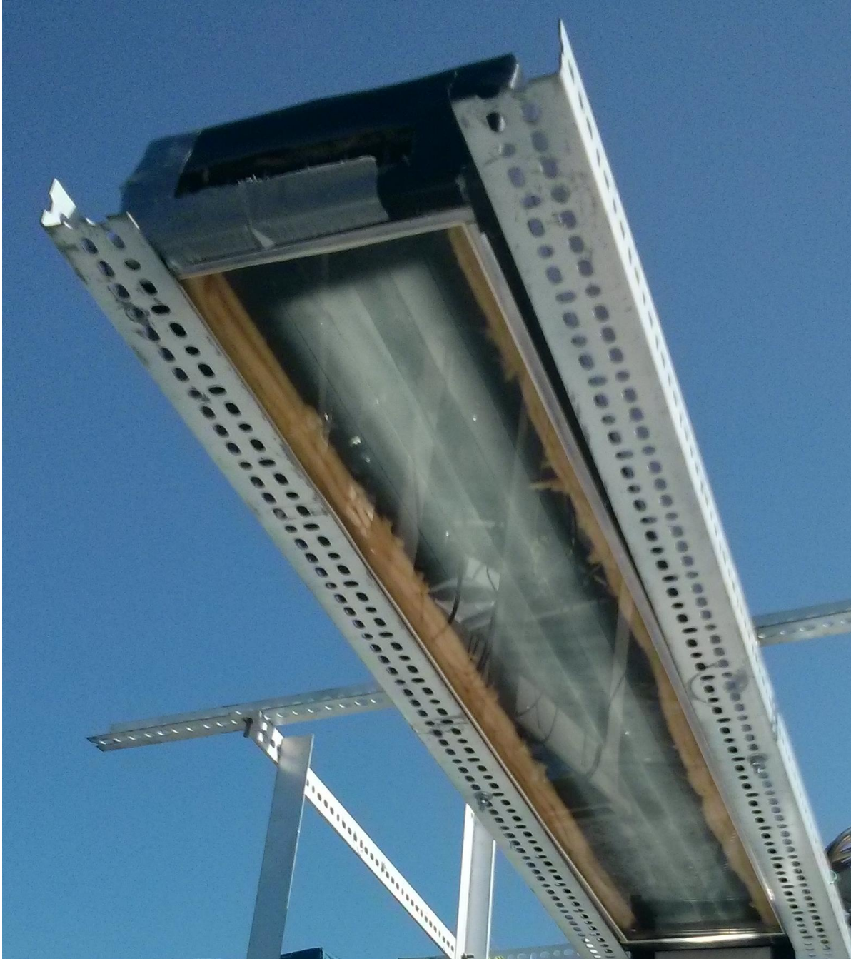
Figure 38: Solar air collector. The image shows the incident radiation that is reflected from the mirrors.
