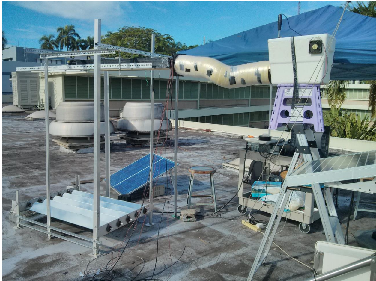
Figure 37: Complete assembly of the Linear Fresnel Reflector System situated in the roof of Stefani Building at the University of Puerto Rico at Mayaguez.
