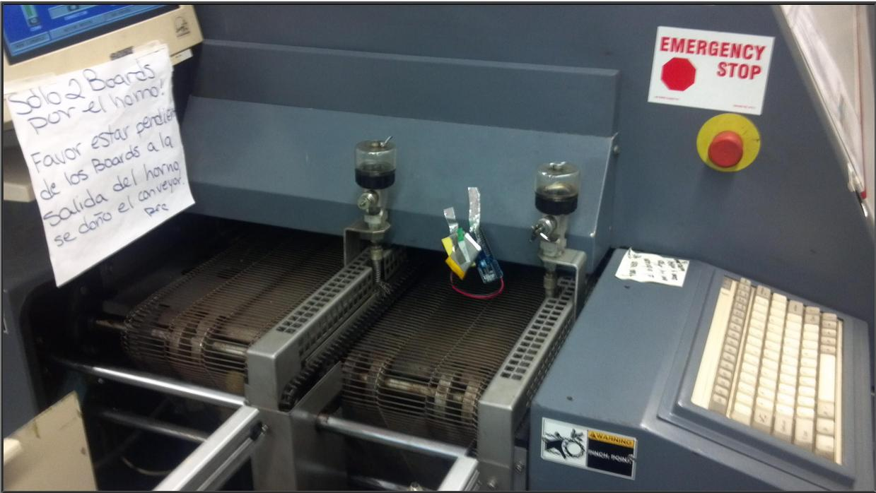
Figure 37: SHT15 node deployment at reflow oven inlet.
