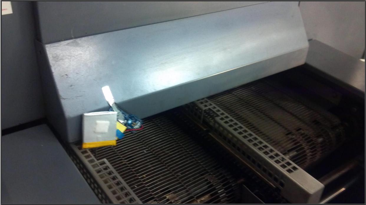
**Figure 38: SHT15 node deployment at reflow oven outlet.**
