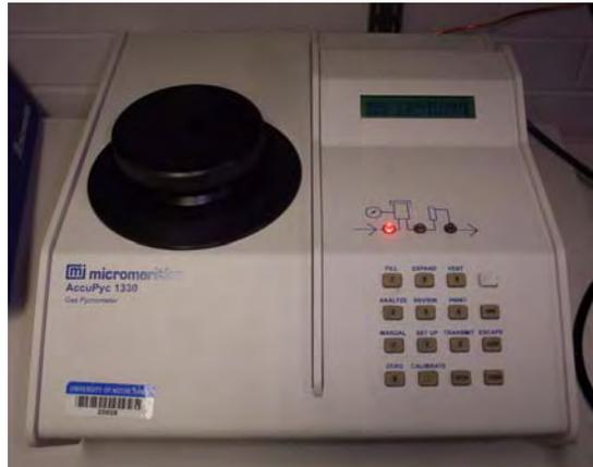
**Figure A.2.3 Micromeritics–AccuPyc 1330 gas pycnometer.
