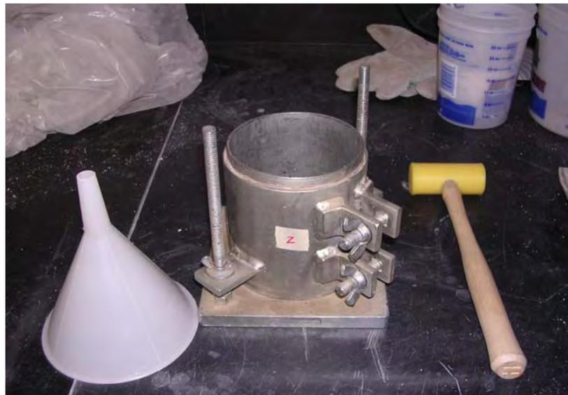
**Figure A.2.2. Alternative method for maximum density test.**
