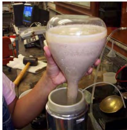
**Figure 3.16. Deposition of calcareous sand using the water pluviation method.**
