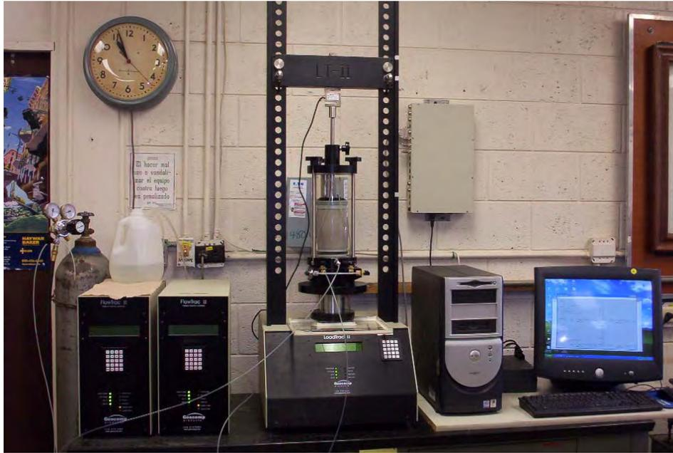
**Figure 3.19. LoadTrac-II/FlowTrac-II Triaxial system, University of Puerto Rico at Mayagüez.**
