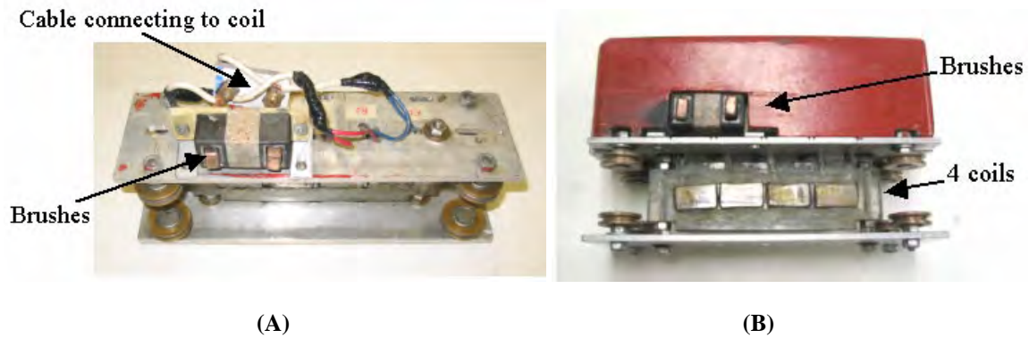
Figure 59: (A) Car with the details of the brushes, (B) Lateral view of the car
