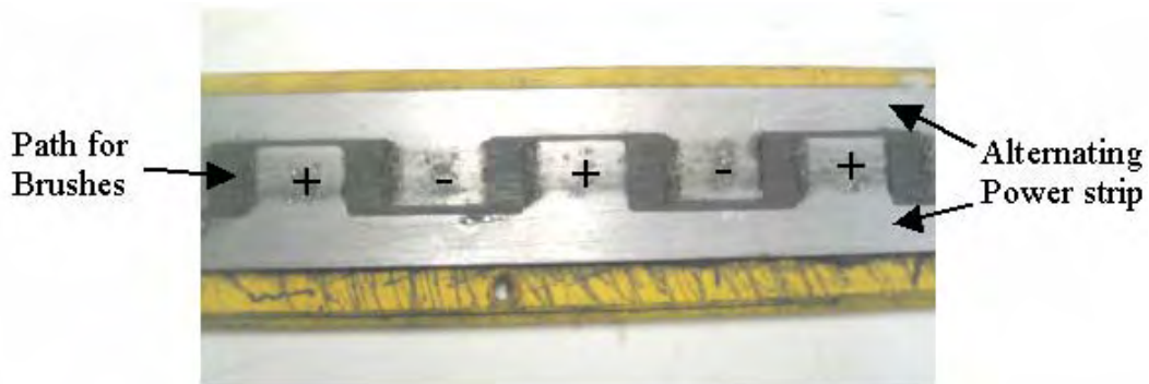
Figure 60: View of the alternating power strip used to power the coils
