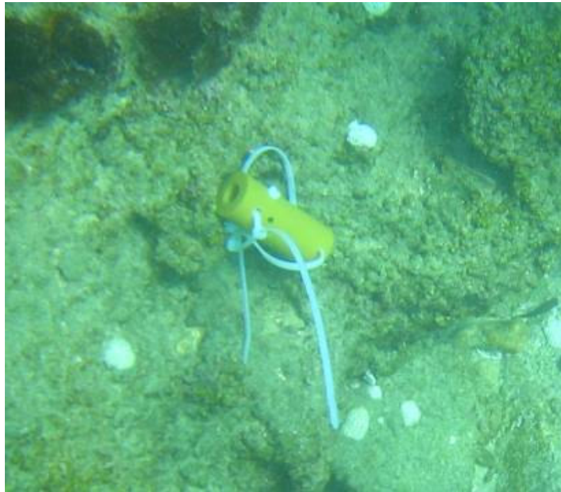
Figure 7.2 Pressure sensor attached to a rock
