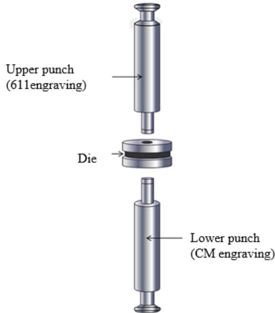
**Figure 4.15** Tablet press upper and lower punches
