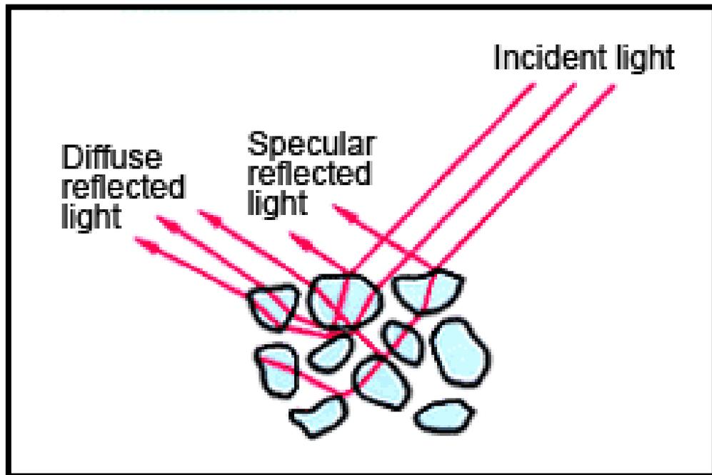
**Figure 2.1** Interaction of the NIR radiation with the tablets particles arise radiation in form of specular reflection and diffuse reflectance. (Image obtained from <http://www.shimadzu.com/an/fir/support/firtalk/talk1/intro.html>)
