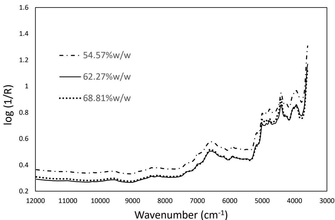
**Figure 4.3** Tablet spectra with three different concentrations of API 54.57, 62.27, and 68.81%w/w.
