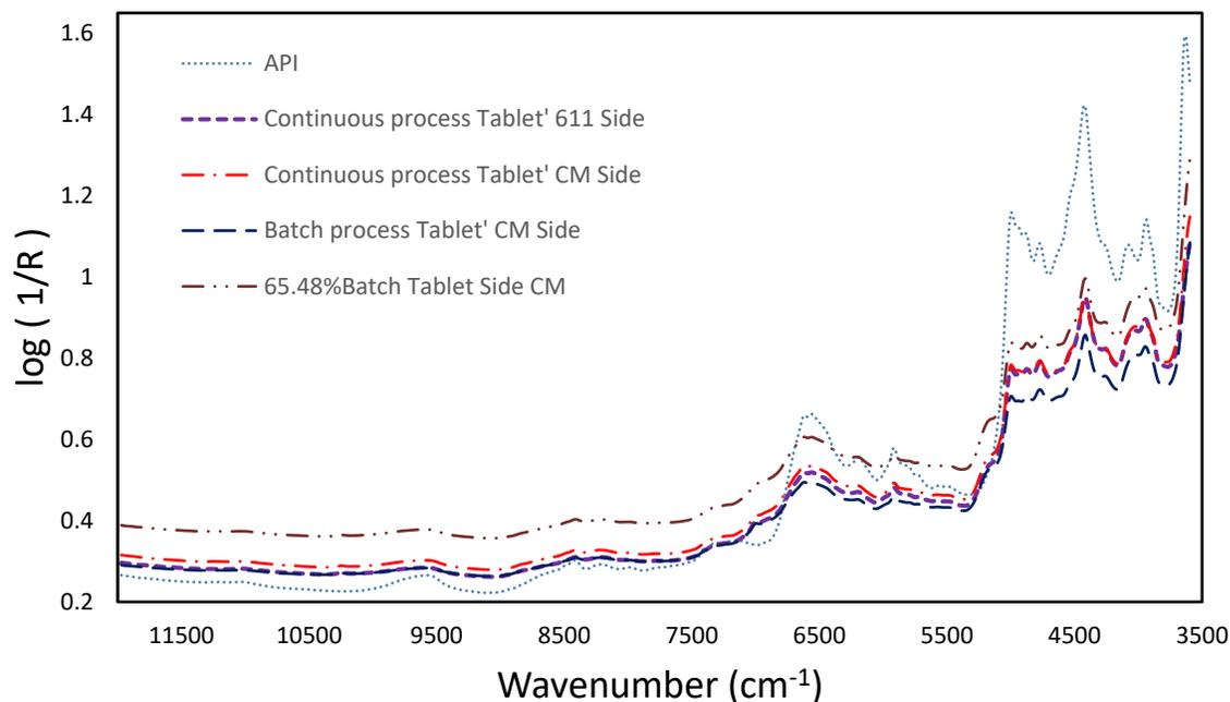
**Figure 4.12** NIR diffuse reflectance spectra of the tablets sides. The spectra of batch tablet with 65.48%(w/w) of API is has a similar API band intensity at  $6,500\text{cm}^{-1}$  with the CM side of the continuous process (test set #2) tablet.
