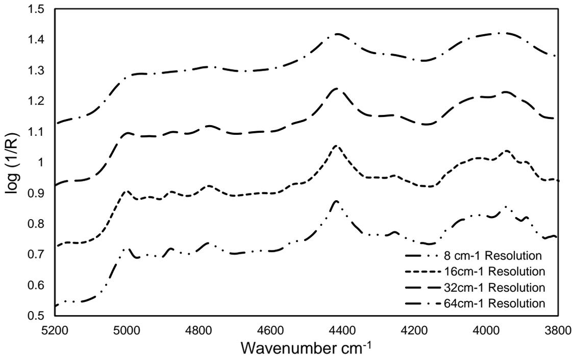
**Figure 4.2** . A comparison between spectra of the same tablet taken at spectral resolution at 8, 16, 32, and 64  $\text{cm}^{-1}$  at 32 scans.
