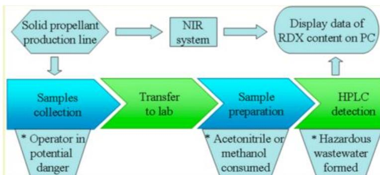
**Figure 1.1** NIR spectroscopy over HPLC as a green chemistry tool in the determination of the hexahydro-1,3,5-trinitro-1,3,5-triazine (RDX) content of a solid propellant.
