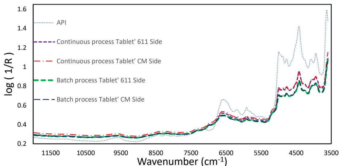
**Figure 4.10** NIR diffuse reflectance spectra of pure API and spectra of the CM and 611 sides of the batch and continuous process tablets (test set #2).
