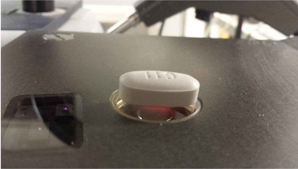
**Figure 3.2** Tablet spectra acquisition illustration using the integrating sphere.
