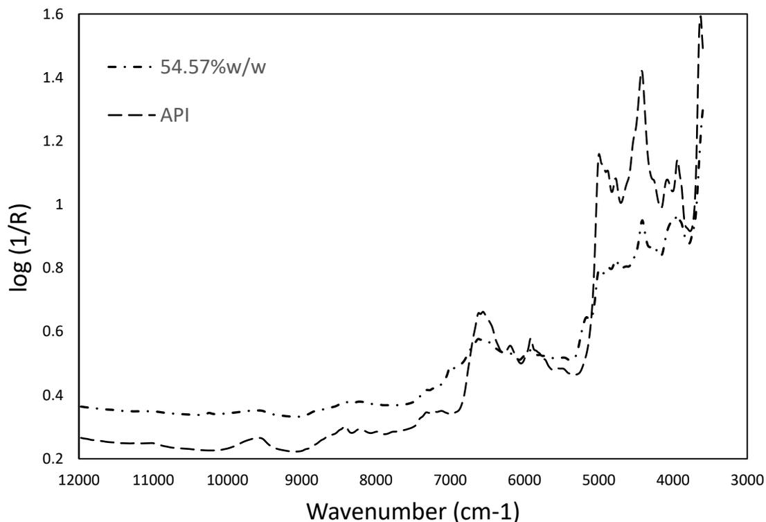
**Figure 4.4.** Pure API spectrum and the tablet spectrum with the lower API concentration
