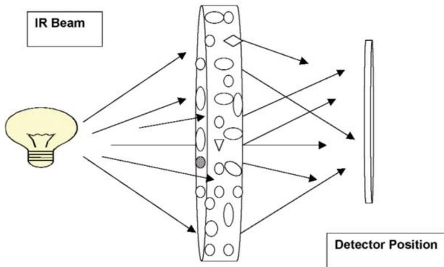
**Figure 2.2** Show the transmittance measurements in a tablet.
