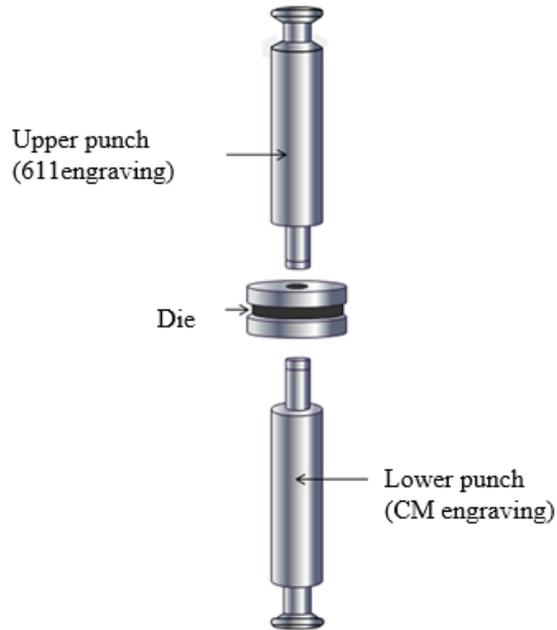
**Figure 4.15** Tablet press upper and lower punches
