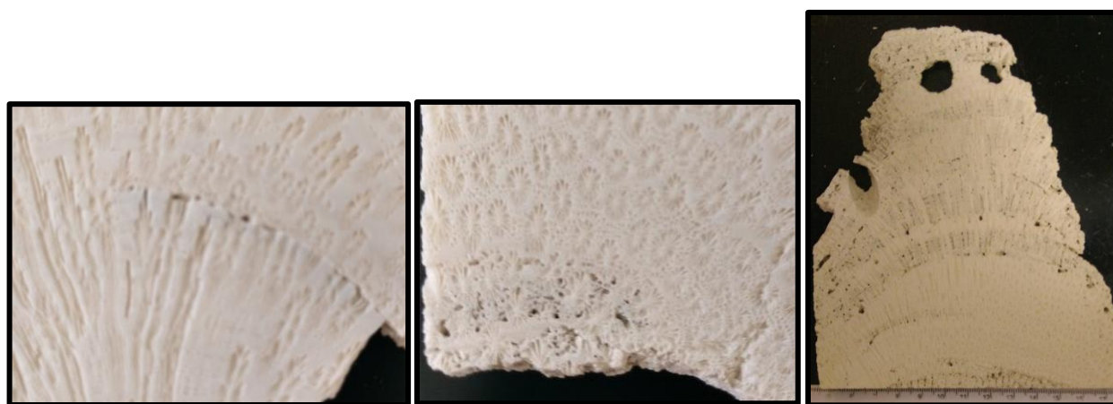
Figure 9. From left to right: Sample M2 150.7-1.3, M2 148-0.6, and M2 120.5-0.4. M2 150.7-1.3. Sample M2 150.7-1.3 shows a surface where growth was discontinuous. M2 148-0.6 shows signs
