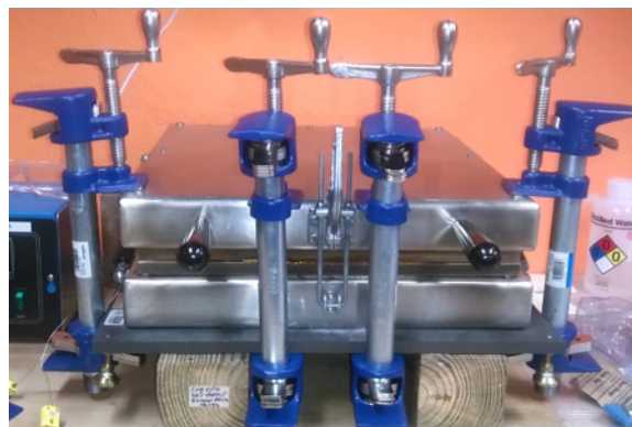
Figure 3. 3. First hot press used to fabricate CNTs/PEEK composites. [49]
