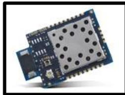
Figure 2-9 Laird Technologies LT2510 FlexRF® 2.4 GHz Wireless Module
